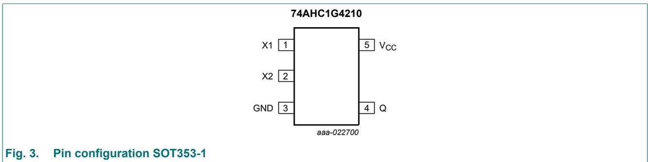
Fig. 3. Pin configuration SOT353-1
