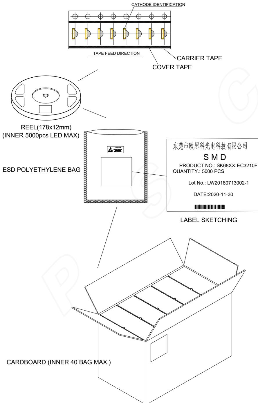
The reel pack is applied in SMD LED. The LEDs are packed in cardboard boxes after packaging in normal or anti-electrostatic bags. cardboard boxes will be used to protect the LEDs from mechanical shocks during transportation. The boxes are not water resistant and therefore must be kept away from water and moisture.
