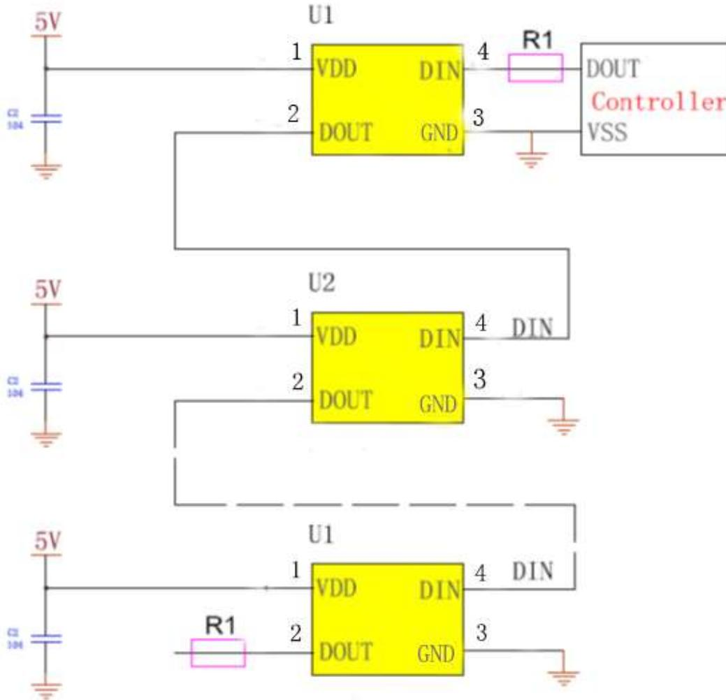
In the practical application circuit, the signal input and output pins of the IC signal input and output pins should be connected to the signal input and output terminals. In addition, in order to make the IC chip is more stable, even the capacitance between beads is essential back;
