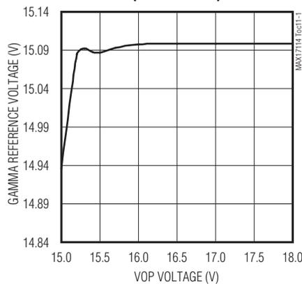
**GAMMA REFERENCE LOAD REGULATION ( $V_{REF} = 16\text{V}$ )**
