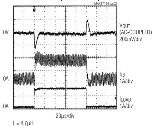
**STEP-DOWN REGULATOR HEAVY-LOAD SOFT-START (1A)**
