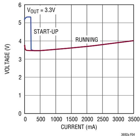
**Figure 4. Minimum Input Voltage vs Load Current**
