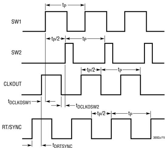
Figure 10. Timing Diagram RT/SYNC = 1MHz, Duty Cycle = 50%
