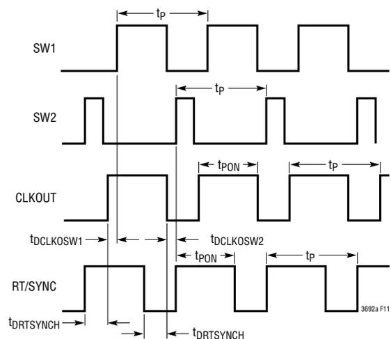
Figure 11. Timing Diagram RT/SYNC = 1MHz, Duty Cycle > 50%
