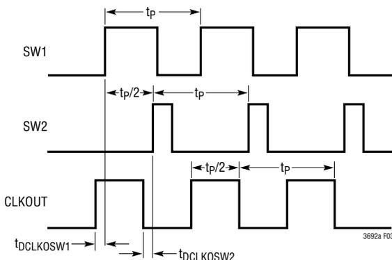
**Figure 3. Timing Diagram RT/SYNC = 28.0k, t<sub>p</sub> = 1μs, V<sub>DIV</sub> = 0V**
