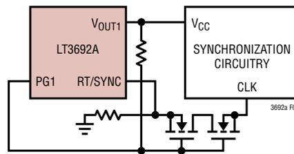
Figure 9. Synchronous Signal Powered from Regulator's Output
