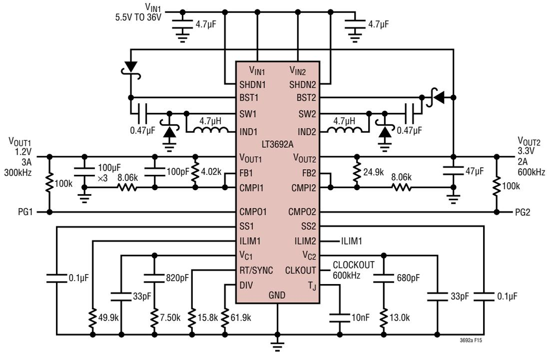
Figure 15. 3.3V and 1.2V Dual Step-Down Multi-Frequency Converter
