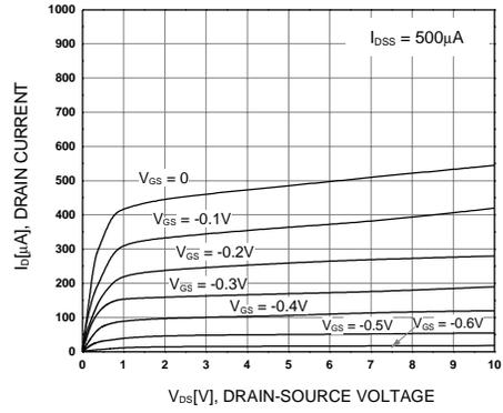
Figure 2.  $I_D$ - $V_{DS}$
