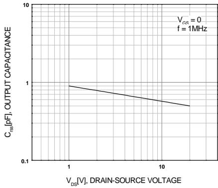
Figure 7.  $C_{RSS}$ - $V_{DS}$
