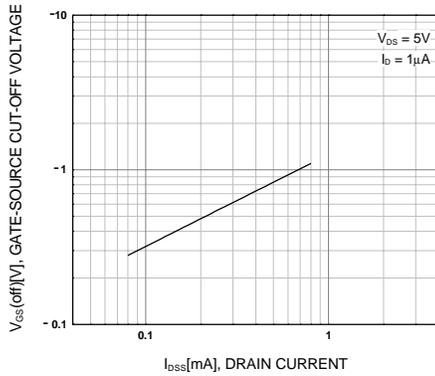
Figure 5.  $V_{GS(off)}$ - $I_{DSS}$
