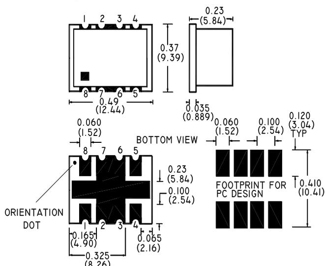
\* Dimensions are inches (millimeters)  $\pm 0.015$  (0.38) unless otherwise specified.
