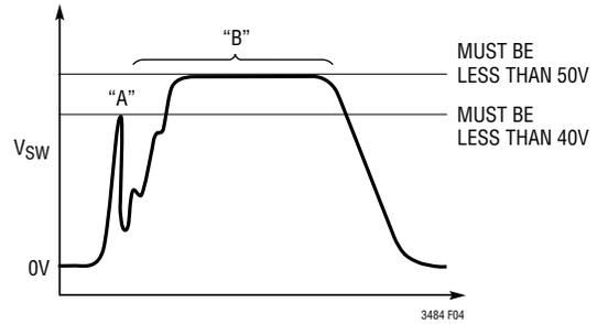
Figure 4. New Transformer Design Check (Not to Scale)
