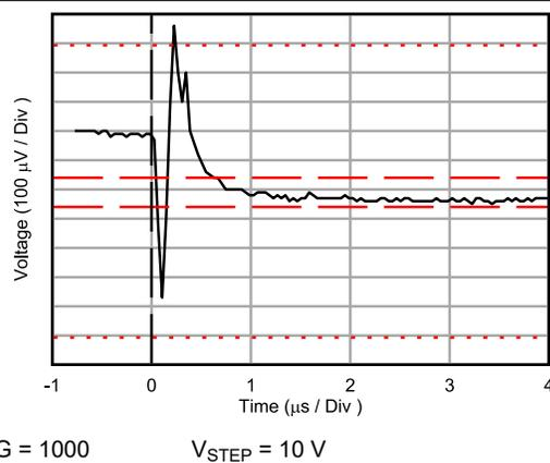
Figure 7-41. Settling Time for  $G = 1000$
