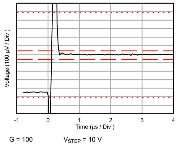
Figure 7-40. Settling Time for  $G = 100$
