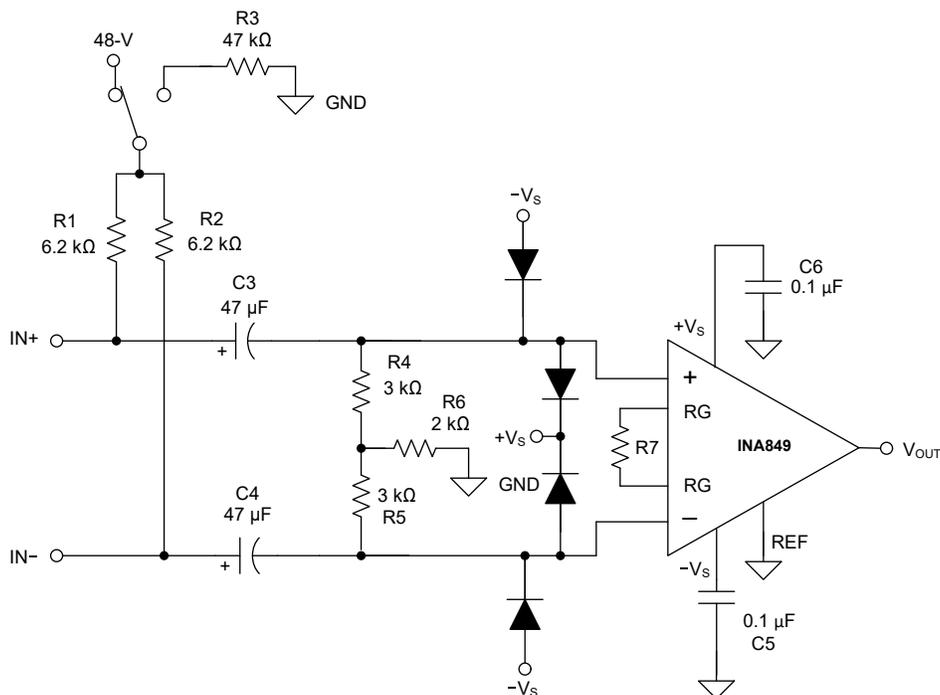
**Figure 9-7. Phantom Power in Microphone Preampifier Circuit**
