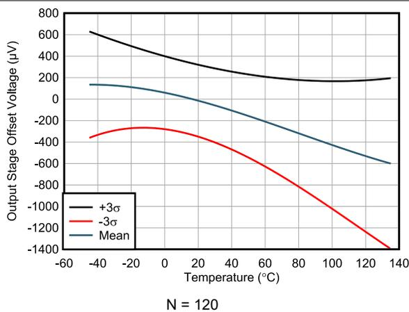
Figure 7-11. Output Stage Offset Voltage vs Temperature
