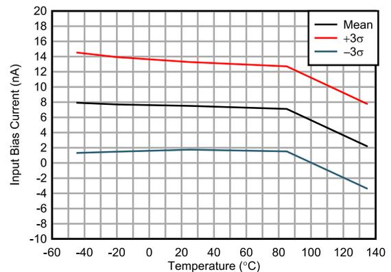
**Figure 7-18. Input Bias Current vs Temperature**
