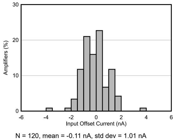
Figure 7-7. Typical Distribution of Input Offset Current
