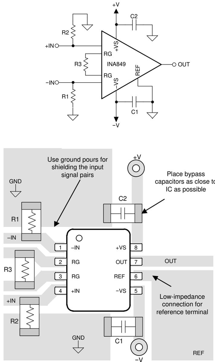
Figure 11-1. Example Schematic and Associated PCB Layout
