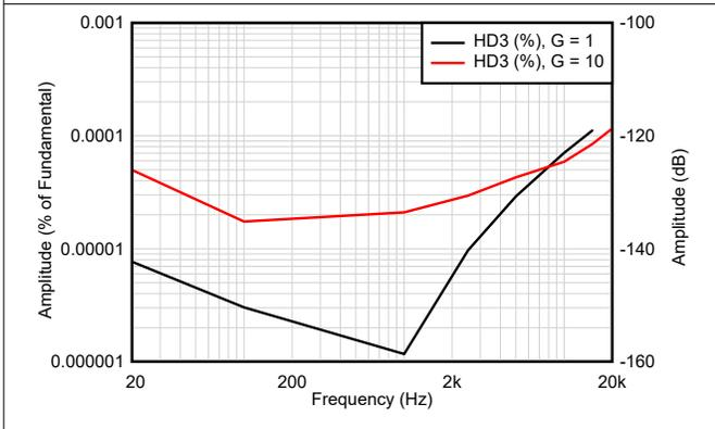
**Figure 7-45. Third Harmonic Distortion vs Frequency**
