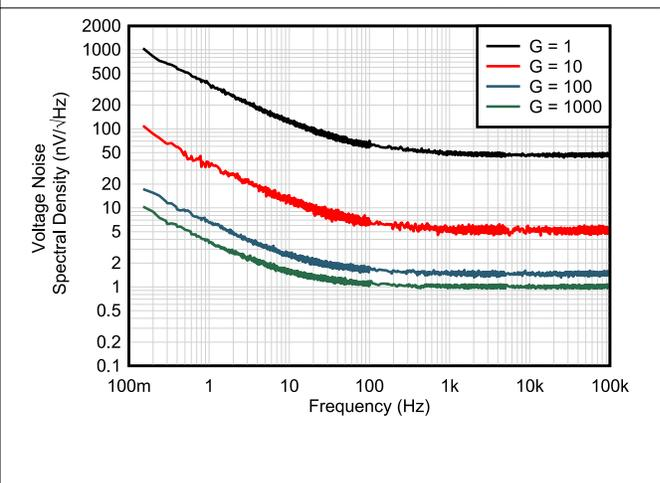
Figure 7-24. Voltage Noise Spectral Density vs Frequency (RTI)
