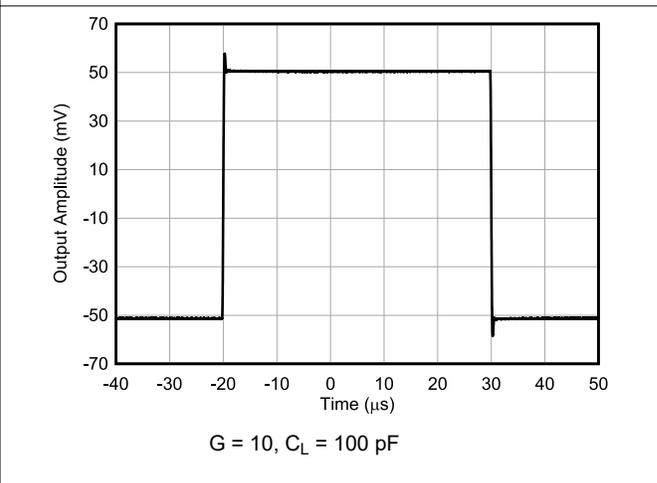
Figure 7-36. Small-Signal Step Response at  $G = 10$
