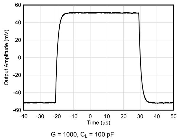
Figure 7-38. Small-Signal Step Response at  $G = 1000$
