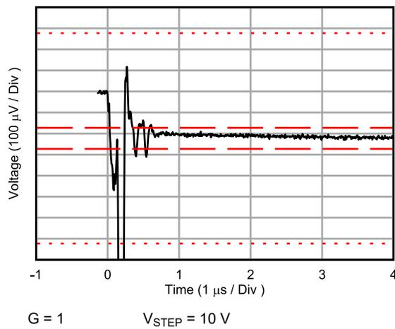
Figure 7-39. Settling Time for  $G = 1$
