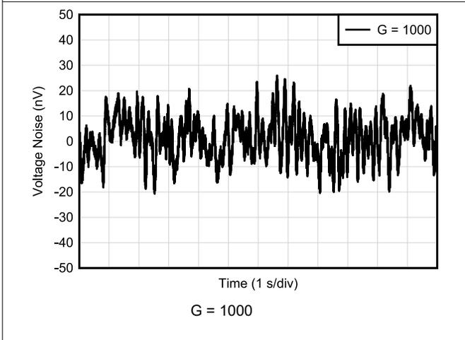
Figure 7-27. 0.1-Hz to 10-Hz RTI Voltage Noise
