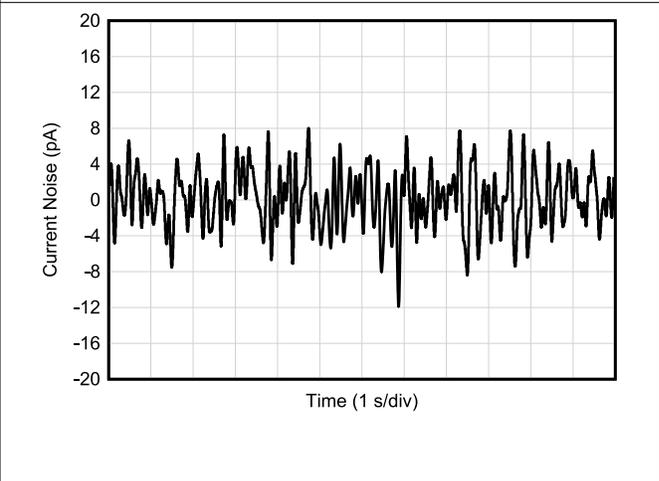
Figure 7-28. 0.1-Hz to 10-Hz RTI Current Noise
