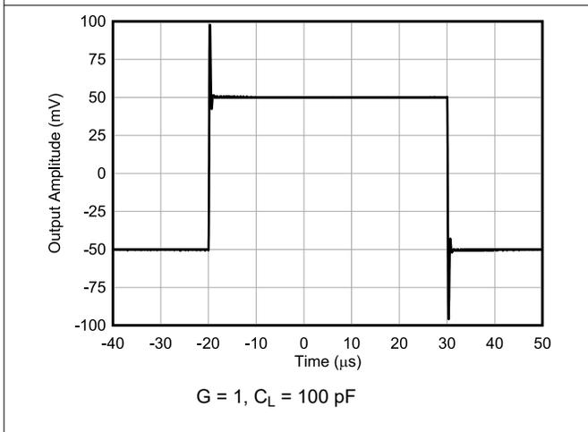
Figure 7-35. Small-Signal Step Response at  $G = 1$
