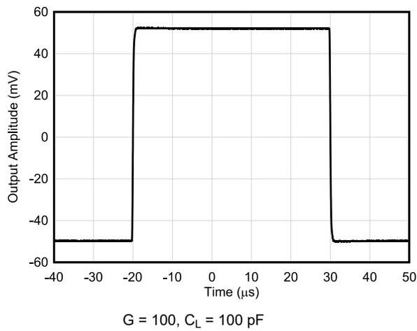
Figure 7-37. Small-Signal Step Response at  $G = 100$
