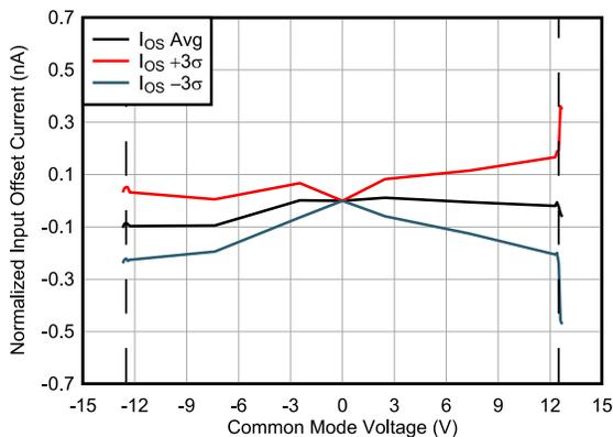
**Figure 7-17. Input Offset Current vs Input Common-Mode Voltage**
