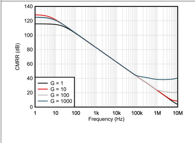
Figure 7-21. CMRR vs Frequency (1-kΩ source imbalance)
