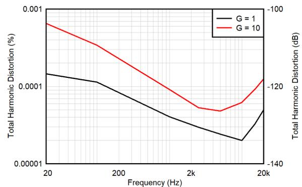
Figure 7-42. Total Harmonic Distortion vs Frequency
