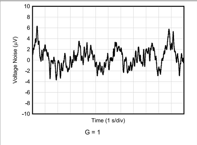
Figure 7-26. 0.1-Hz to 10-Hz RTI Voltage Noise
