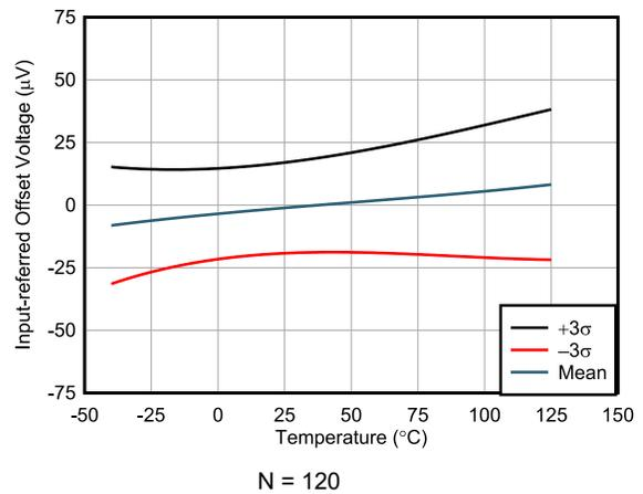
Figure 7-10. Input Stage Offset Voltage vs Temperature
