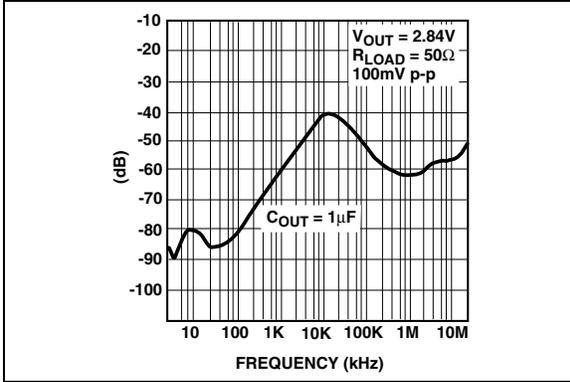
**FIGURE 2-7:** Power Supply Rejection Ratio vs. Frequency. (TC1188)
