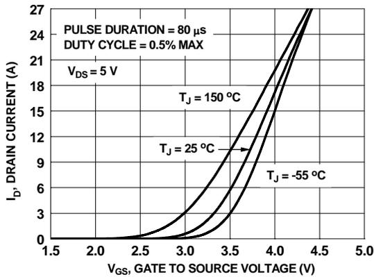
Figure 5. Transfer Characteristics
