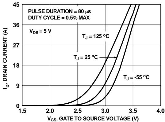
Figure 17. Transfer Characteristics
