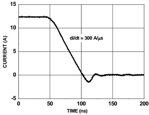
Figure 25. FDMS7620S SyncFET<sup>™</sup> Body Diode Reverse Recovery Characteristic
