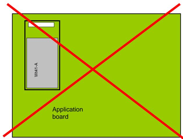
Figure 9: Do not place the module so that the GND plane reaches in front of the antenna
