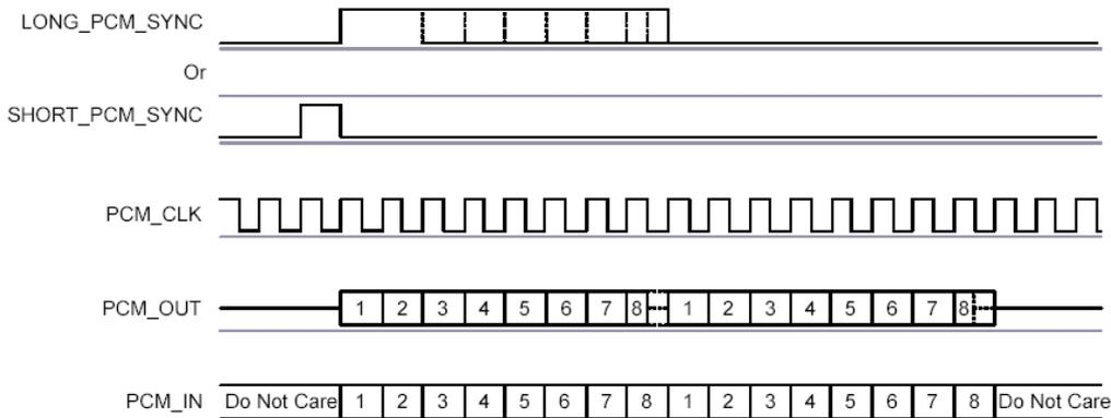
**Figure 23: Multi-slot Operation with Two Slots and 8-bit Companded Samples**
