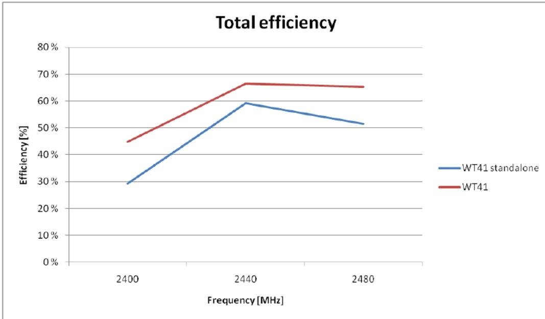
Table 14: Total efficiency of the chip antenna
