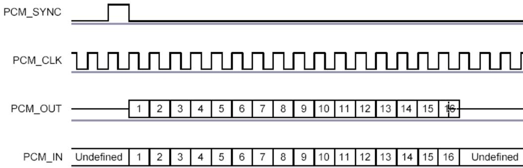
**Figure 22: Short Frame Sync (Shown with 16-bit Sample)**
