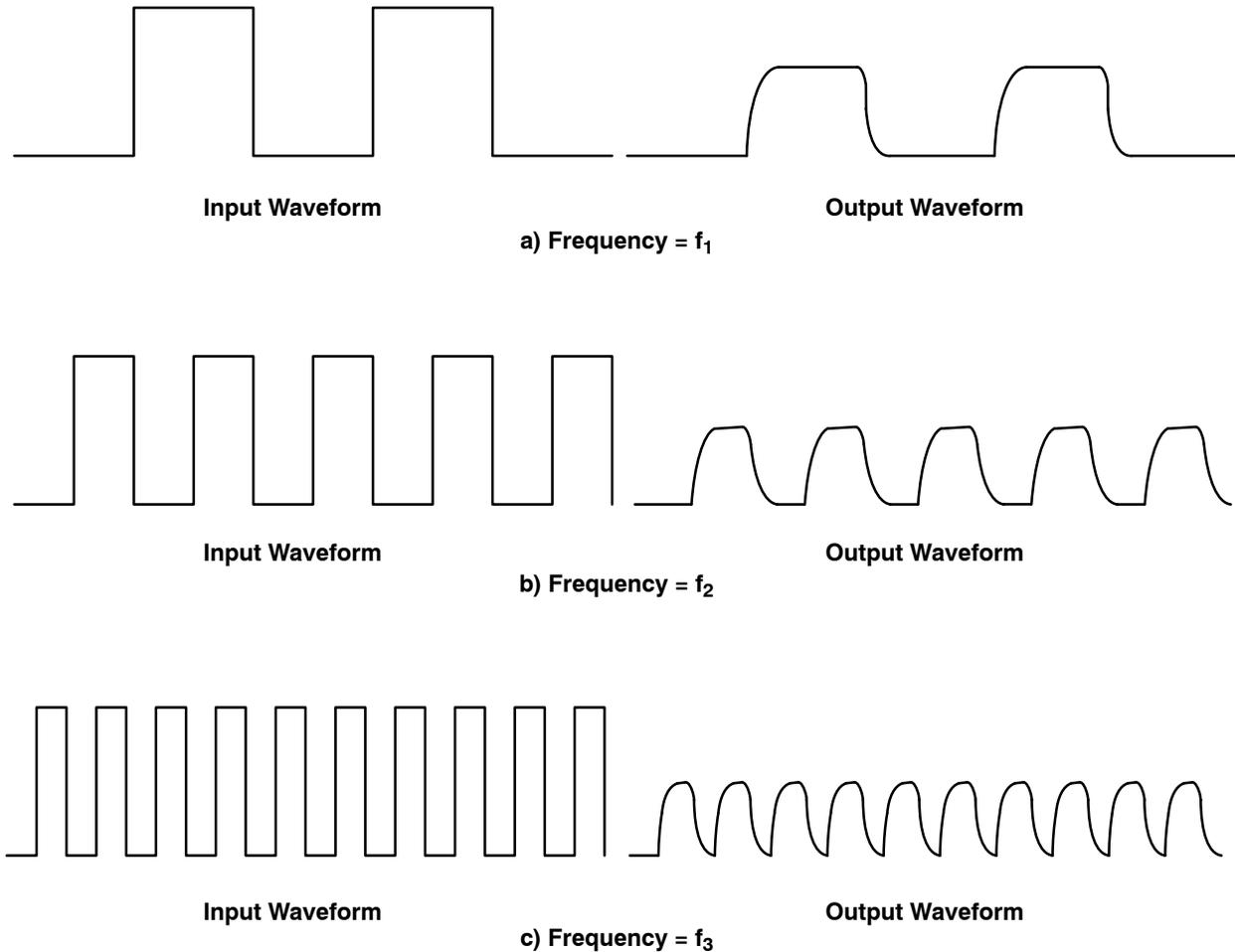
Figure 8. Input and Output Waveforms of Filter
