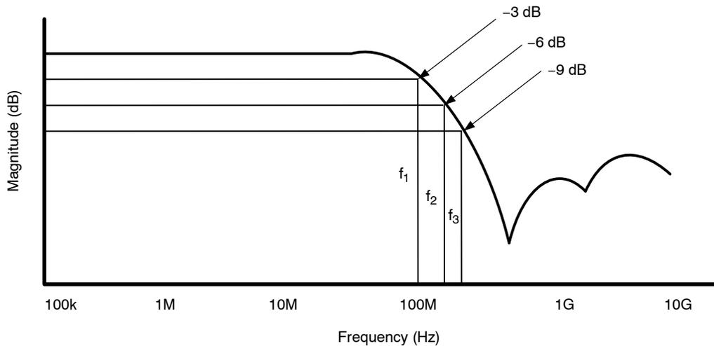
**Figure 7. Filter Bandwidth**
