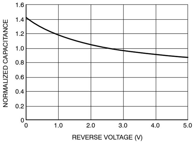
Figure 5. Typical Capacitance
