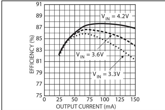
**FIGURE 2-1:** Efficiency at  $V_{OUT} = 12V$ .
