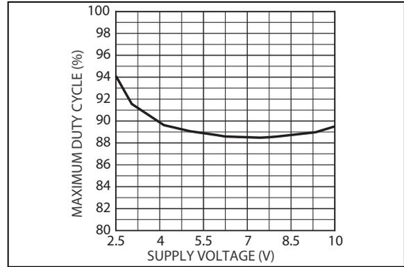
**FIGURE 2-10:** Maximum Duty Cycle vs. Supply Voltage.
