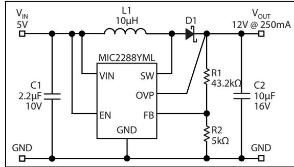
**FIGURE 6-7:** 5V  $V_{IN}$  to 12V  $V_{OUT}$  @ 250 mA.
