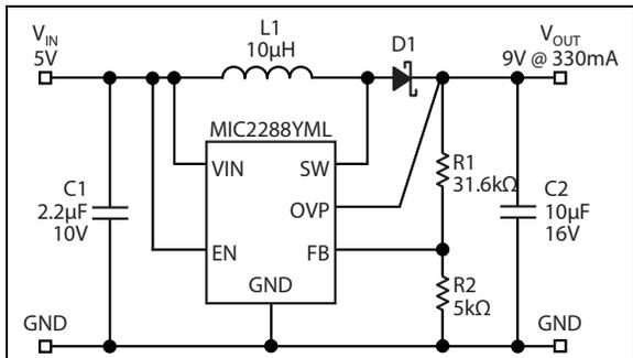
**FIGURE 6-6:** 5V  $V_{IN}$  to 9V  $V_{OUT}$  @ 330 mA.
