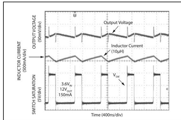
**FIGURE 2-16:** Output Voltage Ripple and Switching Waveforms.
