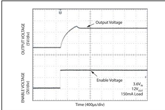
**FIGURE 2-13:** Enable Characteristics.
