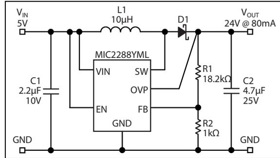
**FIGURE 6-8:** 5V  $V_{IN}$  to 24V  $V_{OUT}$  @ 80 mA.
