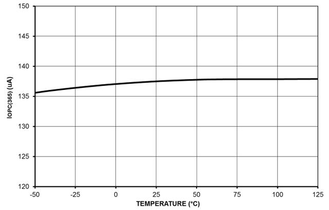
**Figure 40. Current Flowing Out from CS Pin for Over Power Compensation @ 365 V at HV Pin I<sub>OPC(365)</sub>**
