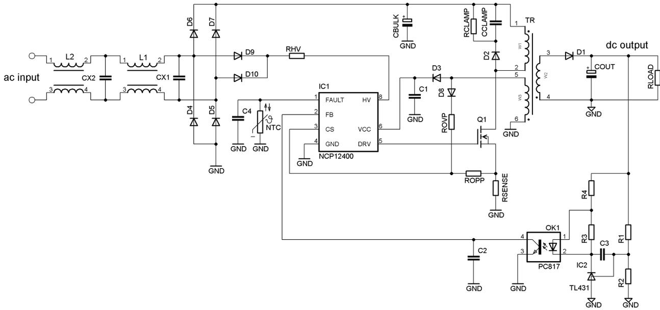
Figure 1. Flyback Converter Application using the NCP12400
