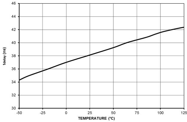
Figure 11. Propagation Delay  $t_{delay}$
