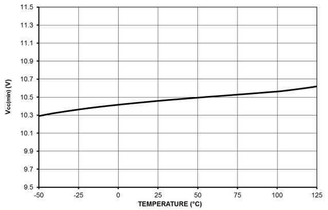
**Figure 29. HV Current Source Restart Threshold V<sub>CC(min)</sub>**
