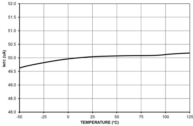
**Figure 39. Current I<sub>NTC</sub> Sourced Out from the Fault Pin, allowing Direct NTC Connection**
