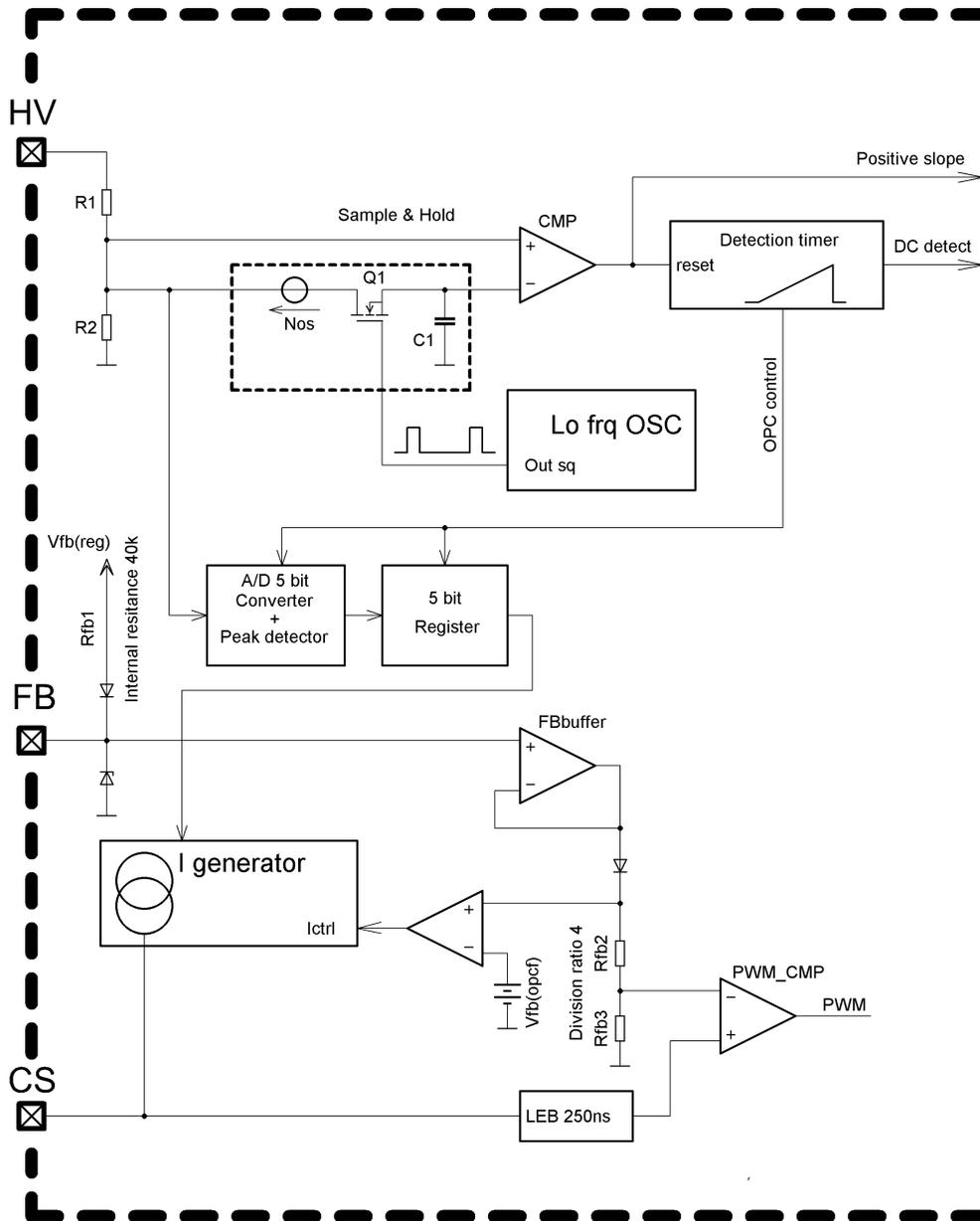
Figure 70. Block Schematic of Overpower Protection Circuit
