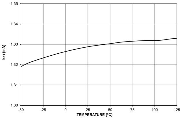
**Figure 28. Internal Current Consumption when DRV Pin is Unloaded I<sub>CC1</sub>**
