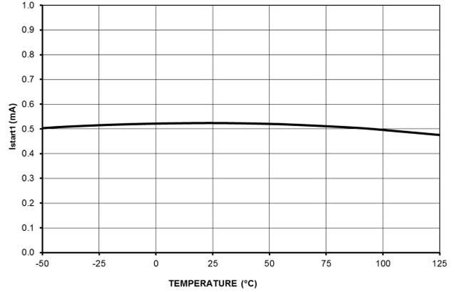
Figure 4. High Voltage Startup Current Flowing Out of V<sub>CC</sub> Pin I<sub>start1</sub> of V<sub>CC</sub> Pin Fault/Short
