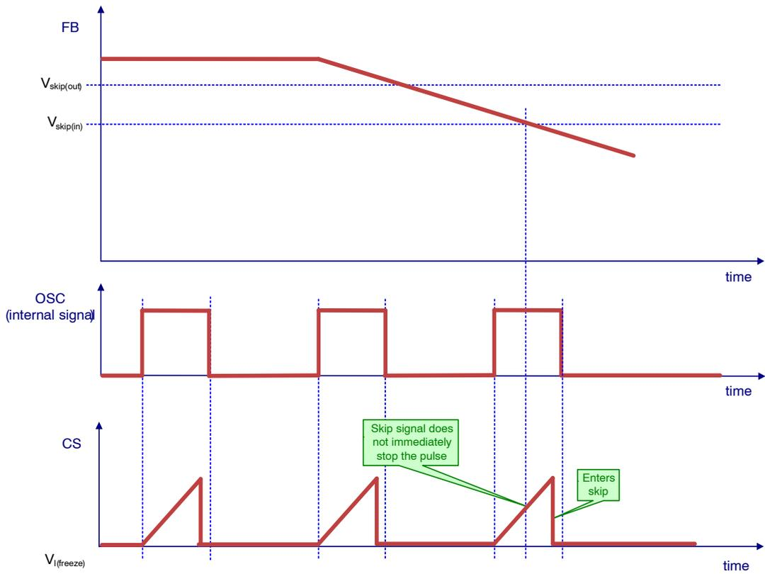
Figure 61. Technique Preventing Short Pulses in Skip Mode
