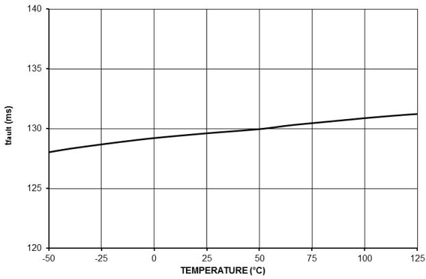
Figure 24. The Fault Timer Duration  $t_{fault}$
