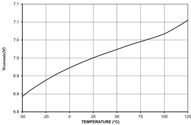
**Figure 30. V<sub>CC</sub> Decreasing Level at which the Internal Logic Resets V<sub>CC(reset)</sub>**
