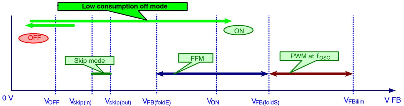
Figure 43. Mode Control with FB Pin Voltage
