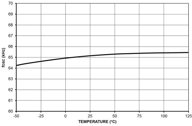
Figure 20. Oscillator Switching Frequency  $f_{osc}$
