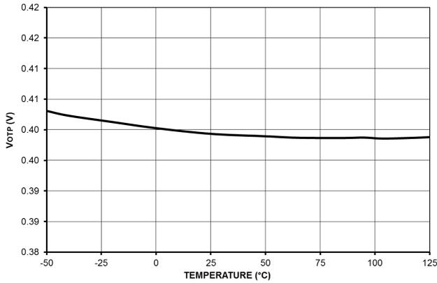
**Figure 41. Fault Pin Low Threshold for OTP V<sub>OTP</sub>**
