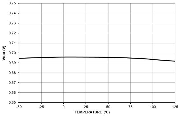
Figure 9. Maximum Internal Current Setpoint  $V_{ILIM}$
