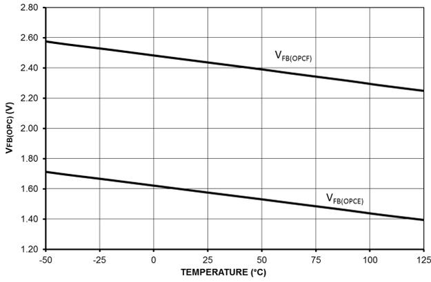
**Figure 37. FB Pin Voltage Thresholds for Overpower Compensation**
