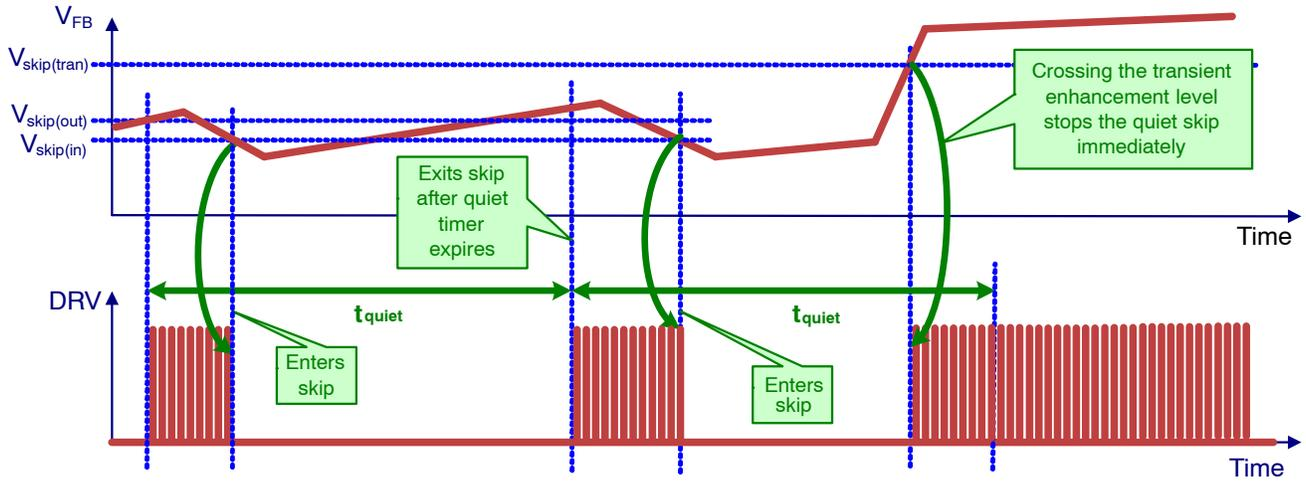
Figure 62. Leaving the Quiet-Skip Mode during Load Transient
