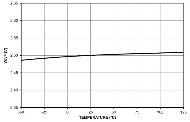
**Figure 38. Fault Pin High Threshold for OVP V<sub>OVP</sub>**
