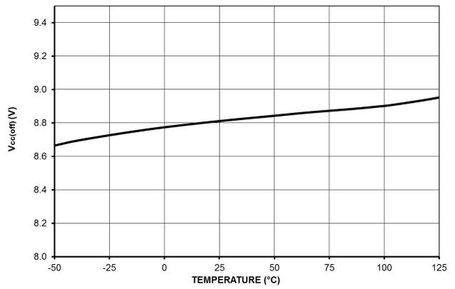
**Figure 27. V<sub>CC</sub> Turn-off Threshold (UVLO) V<sub>CC(off)</sub>**
