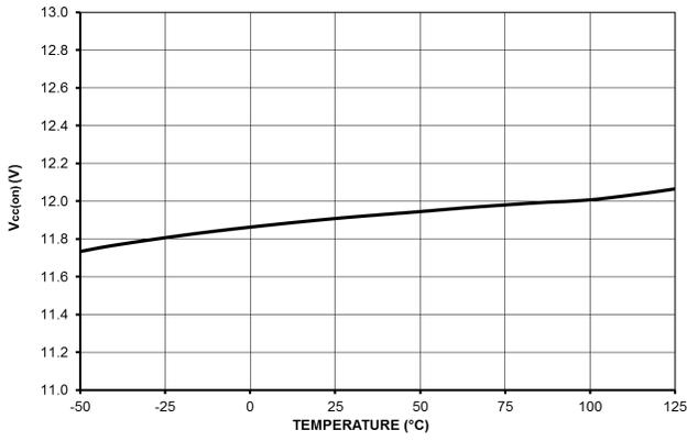
**Figure 26. V<sub>CC</sub> Turn-on Threshold Level, V<sub>CC</sub> Going Up HV Current Source Stop Threshold V<sub>CC(on)</sub>**
