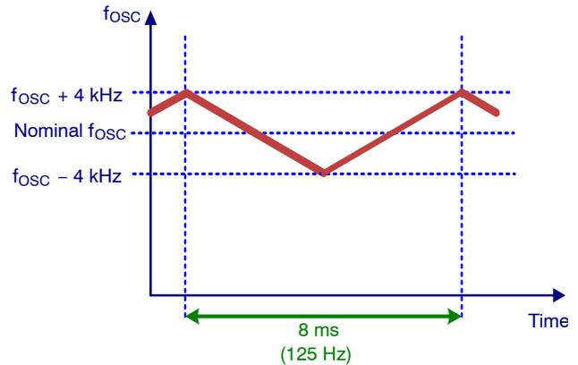
Figure 57. Frequency Modulation of the Maximum Switching Frequency
