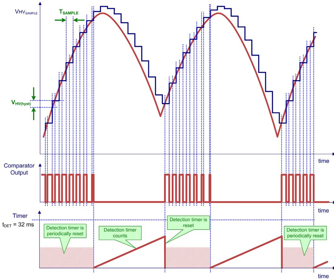
Figure 52. The ac Line Unplug Detector Timing Diagram
