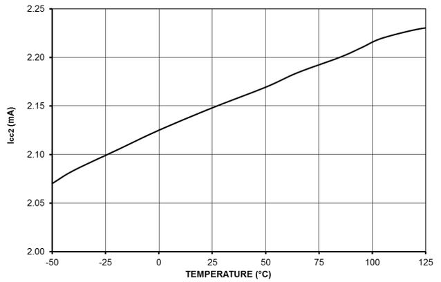
**Figure 31. Internal Current Consumption when DRV Pin is Loaded by 1 nF Capacitance I<sub>CC2</sub>**
