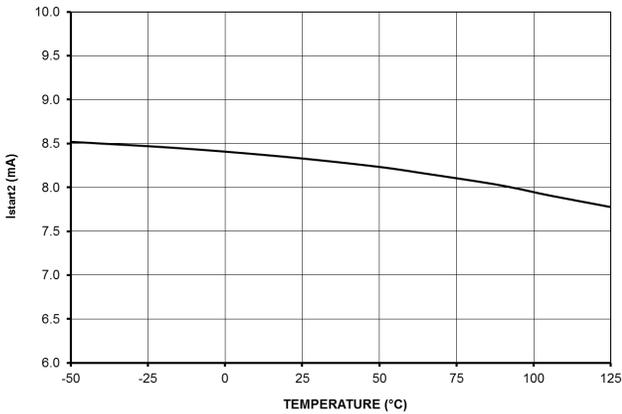
Figure 7. High Voltage Startup Current Flowing Out of V<sub>CC</sub> Pin I<sub>start2</sub>
