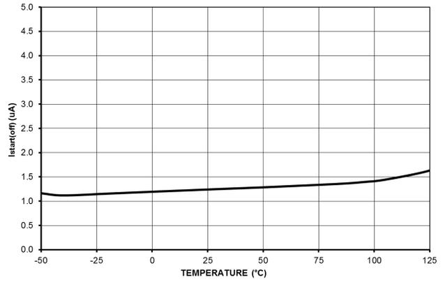
Figure 6. Off-state Leakage Current from HV Pin I<sub>start(off)</sub>
