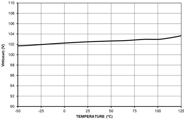
Figure 5. HV Pin Device Startup Threshold V<sub>HV(start)</sub>
