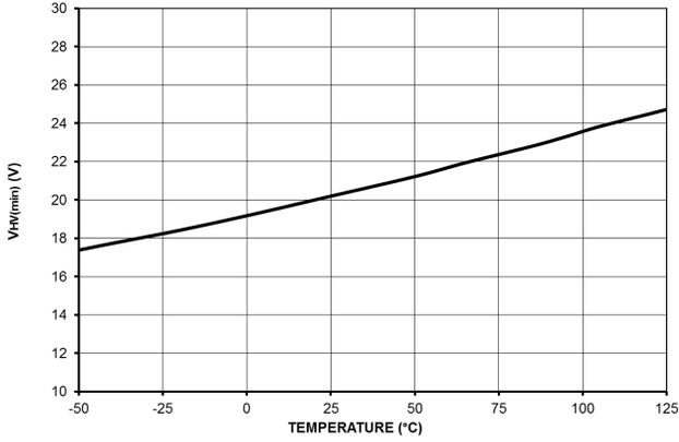
Figure 3. Minimum Voltage for HV Current Source Operation V<sub>HV(min)</sub>
