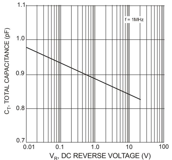
Fig. 4 Typical Total Capacitance vs. Reverse Voltage
