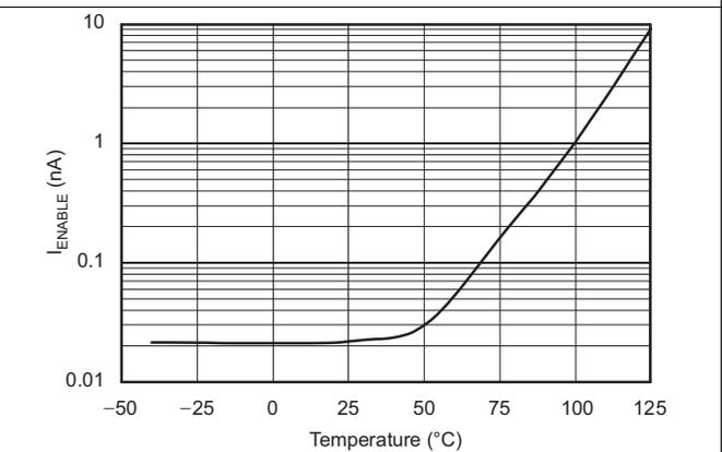
Figure 24.  $I_{ENABLE}$  vs Temperature
