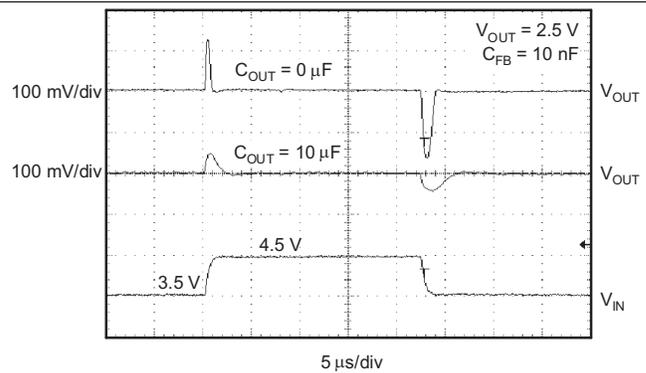
Figure 28. TPS73101 Line Transient, Adjustable Version
