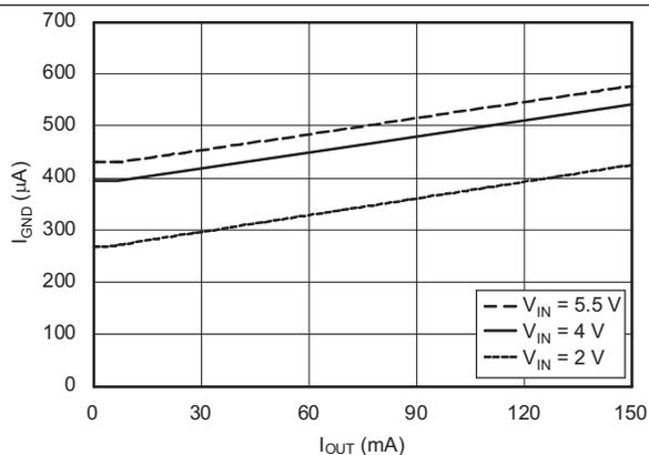
**Figure 7. Ground Pin Current vs Output Current**
