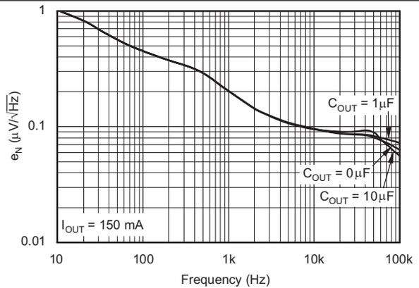
Figure 16. Noise Spectral Density  $C_{NR} = 0.01\text{ }\mu\text{F}$
