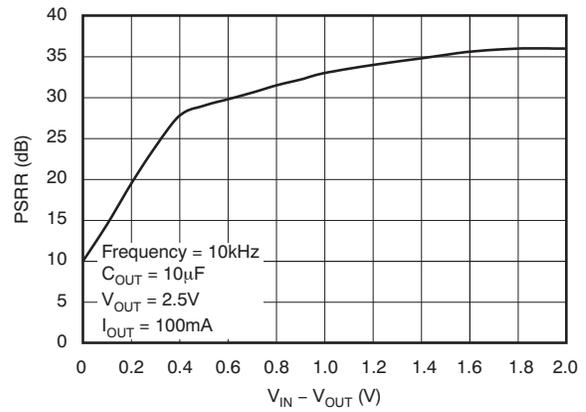
Figure 14. PSRR (Ripple Rejection) vs  $V_{IN} - V_{OUT}$
