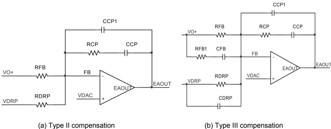
**Figure 21 Voltage loop compensation network**
