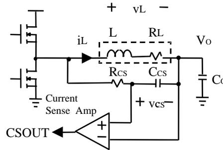
**Figure 7 Inductor Current Sensing and Current Sense Amplifier**
