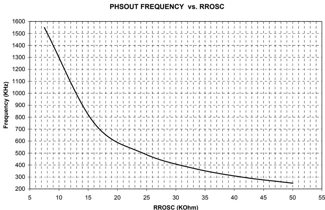
**Figure 2 - Phout Frequency vs. RROSC chart**
