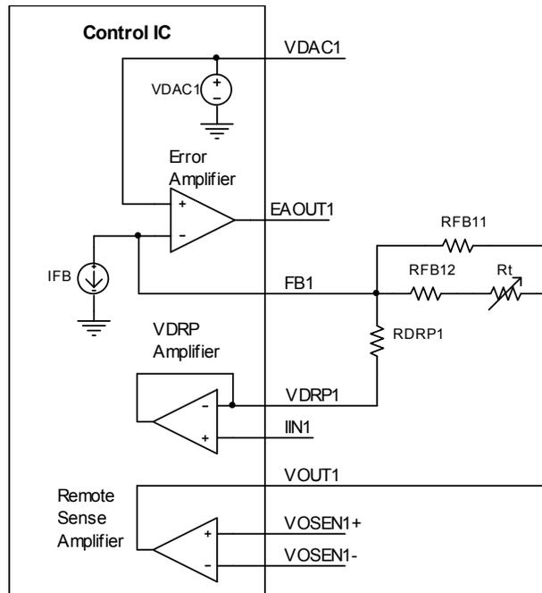
**Figure 10 Temperature compensation of Output1 inductor DCR**
