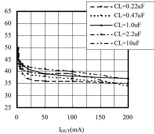
■ Output Noise Level(1/f) vs. Frequency
