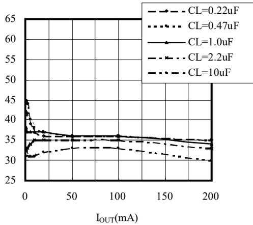
■ Output Noise vs. Output Current
