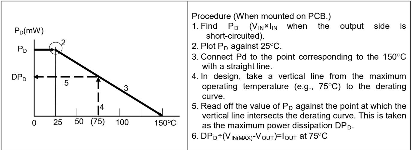
Figure 5. The simple method to calculate PD
