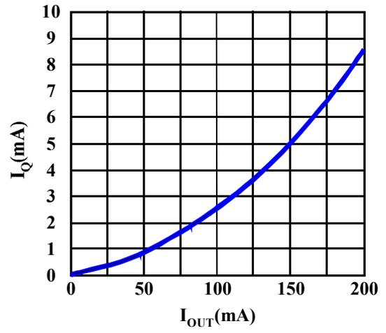
■ Standby Current ( $V_{CONT}=0V$ )
