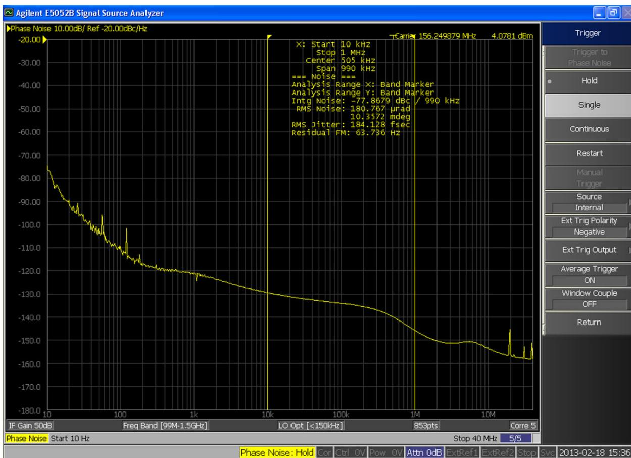
**Figure 1. Si535/536 Typical Phase Noise at 156.25 MHz**
