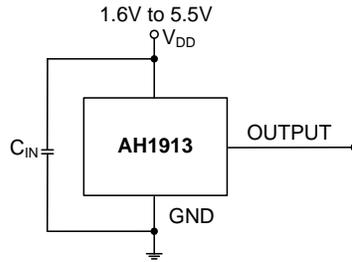
Note: 4.  $C_{IN}$  is for power stabilization and to strengthen the noise immunity; the recommended capacitance is 100nF typical and should be placed as close to the supply pin as possible.
