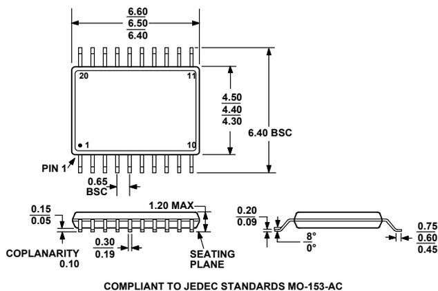
Figure 32. 20-Lead Thin Shrink Small Outline Package [TSSOP]
