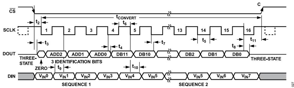
Figure 27. Writing to Shadow Register Timing Diagram
