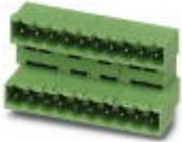
Header, Nominal current: 10 A, Rated voltage (III/2): 320 V, Number of positions: 11, Pitch: 5 mm, Color: green, Contact surface: Tin, Assembly: Soldering, The article can be aligned to create different nos. of positions! In combination with MVSTB or FKCV plug components, both an MVSTBW (or FKCVW) and an MVSTBR plug (or FKCVR) must be used. Combination with TMSTBP plug components is not possible!
