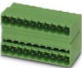
Header, Nominal current: 10 A, Rated voltage (III/2): 320 V, Number of positions: 11, Pitch: 5 mm, Color: green, Contact surface: Tin, Assembly: Soldering, In combination with MVSTB or FKCV plug components, both an MVSTBW (or FKCVW) and an MVSTBR plug (or FKCVR) must be used. Combination with TMSTBP plug components is not possible!
