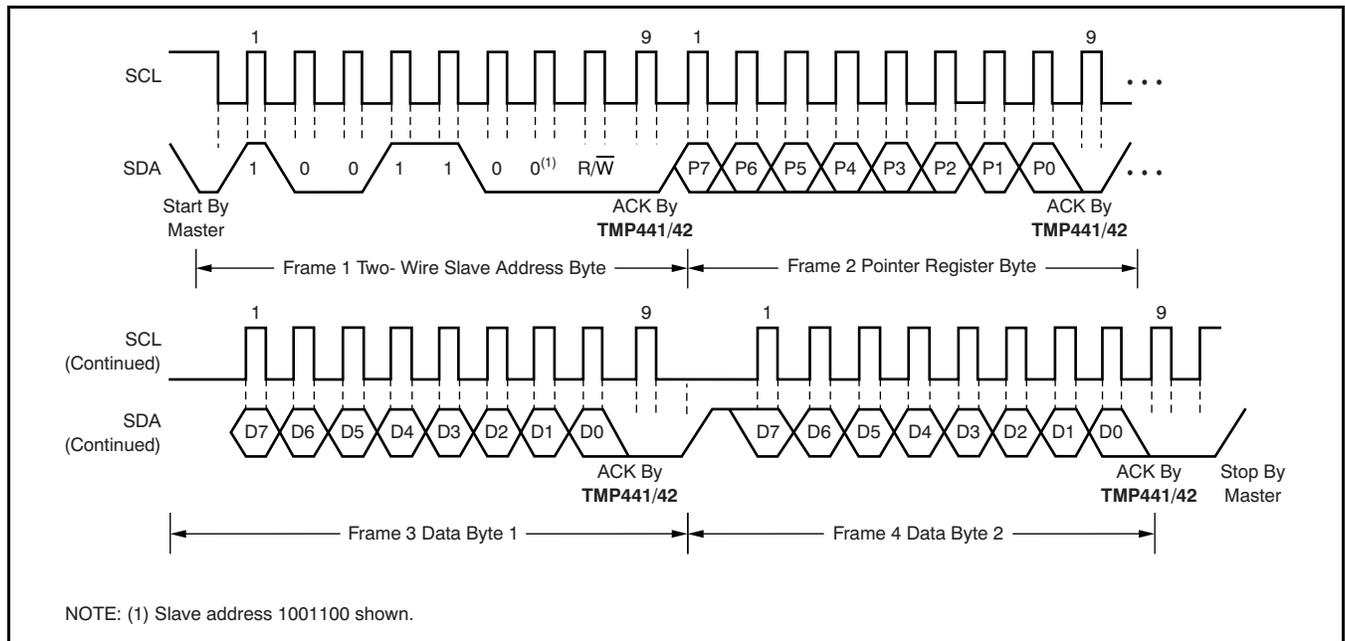
Figure 16. Two-Wire Timing Diagram for Write Word Format
