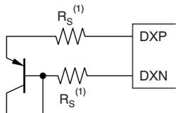
(1)  $R_S$  should be less than 1k $\Omega$ ; see [Filtering](#) section.
