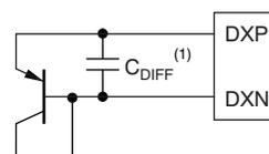
(1)  $C_{DIFF}$  should be less than 300pF; see [Filtering](#) section.
