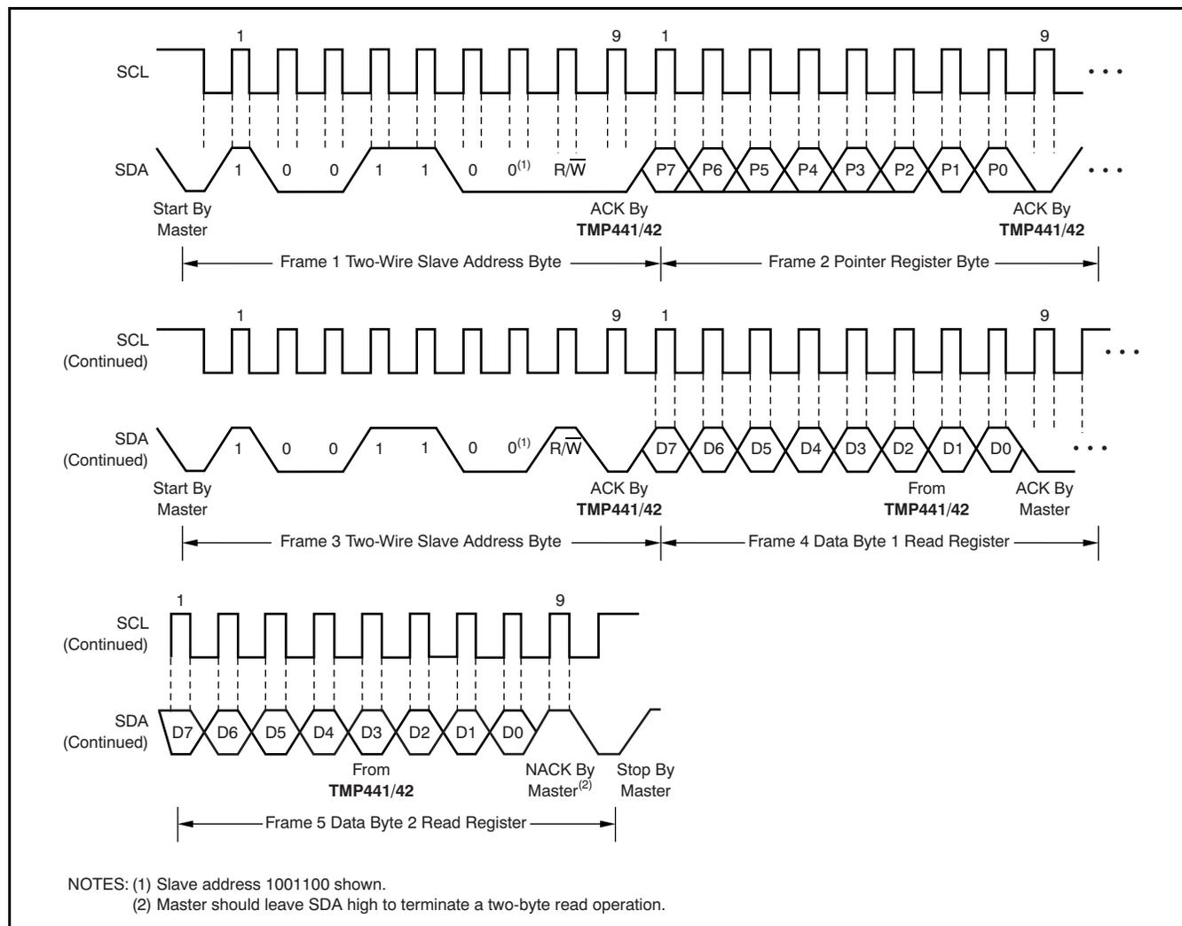
Figure 18. Two-Wire Timing Diagram for Two-Byte Read Format
