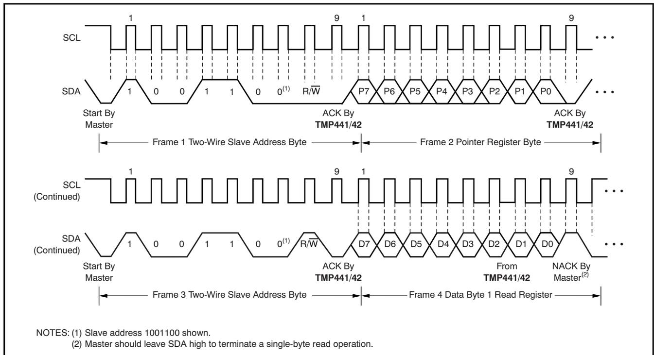
Figure 17. Two-Wire Timing Diagram for Single-Byte Read Format
