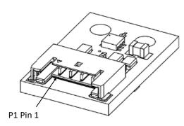
P1—Molex connector P/N 504050-0491 Molex matting connector P/N 5040510401 with terminals 5040520098
