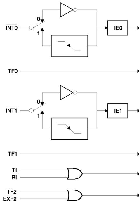
The Timer 0 and Timer 1 flags, TF0 and TF1, are set at S5P2 of the cycle in which the timers overflow. The values are then polled by the circuitry in the next cycle. However,
