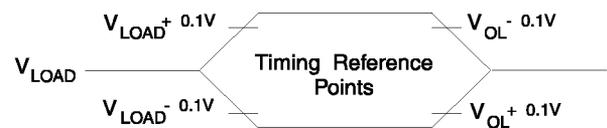
Note: 1. For timing purposes, a port pin is no longer floating when a 100 mV change from load voltage occurs. A port pin begins to float when a 100 mV change from the loaded  $V_{OH}/V_{OL}$  level occurs.
