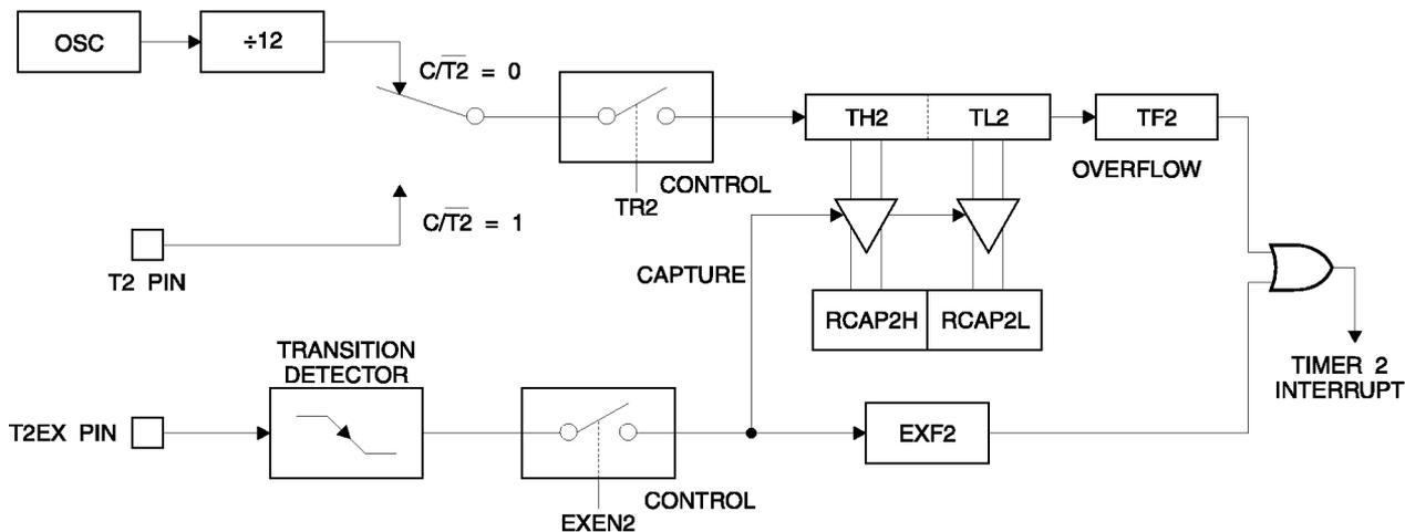
show a high in one cycle and a low in the next cycle, the count is incremented. The new count value appears in the register during S3P1 of the cycle following the one in which the transition was detected. Since two machine cycles (24 oscillator periods) are required to recognize a 1-to-0 transition, the maximum count rate is 1/24 of the oscillator frequency. To ensure that a given level is sampled at least once before it changes, the level should be held for at least one full machine cycle.
