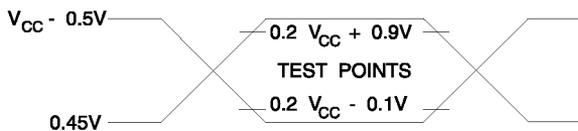
Note: 1. AC Inputs during testing are driven at  $V_{CC} - 0.5V$  for a logic 1 and  $0.45V$  for a logic 0. Timing measurements are made at  $V_{IH}$  min. for a logic 1 and  $V_{IL}$  max. for a logic 0.
