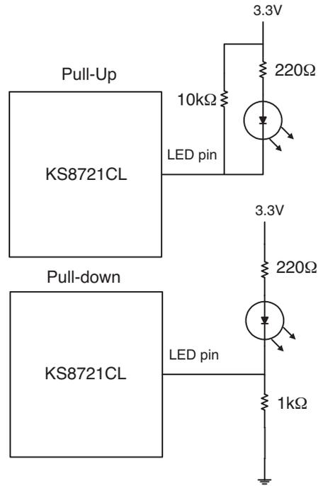
Reference circuits for unmanaged programming through LED ports
