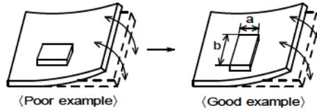
(2) Components location on PCB separation
