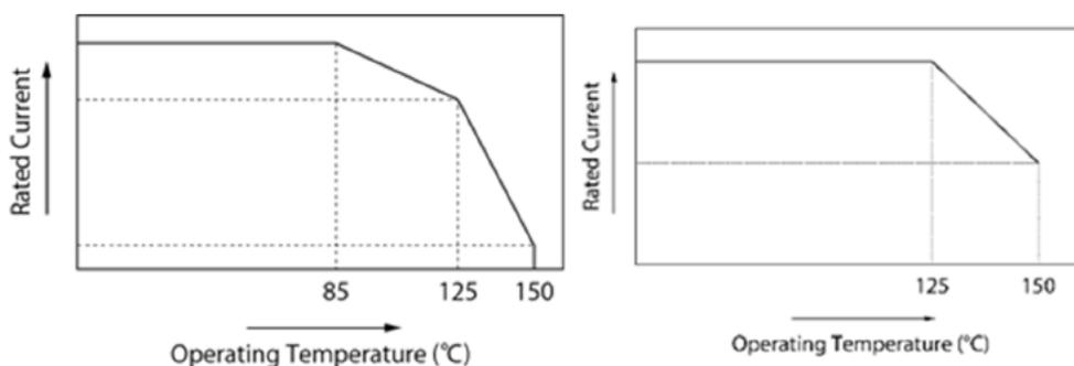
\*2 Keep the temperature (ambient temperature plus self-generation of heat) under 155°C.
