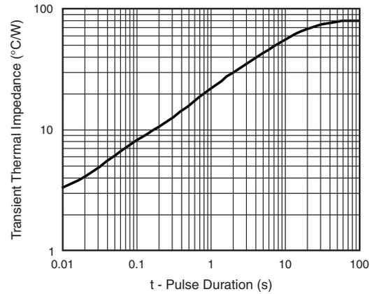
Fig. 6 - Typical Transient Thermal Impedance Per Leg
