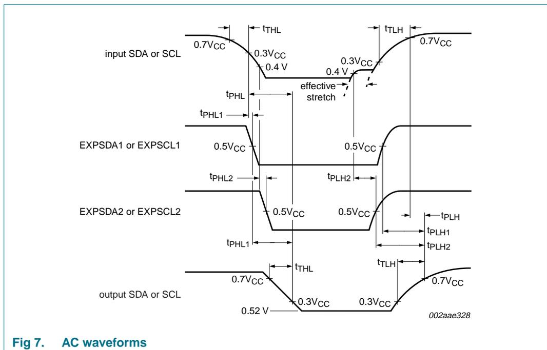
**Fig 7. AC waveforms**
