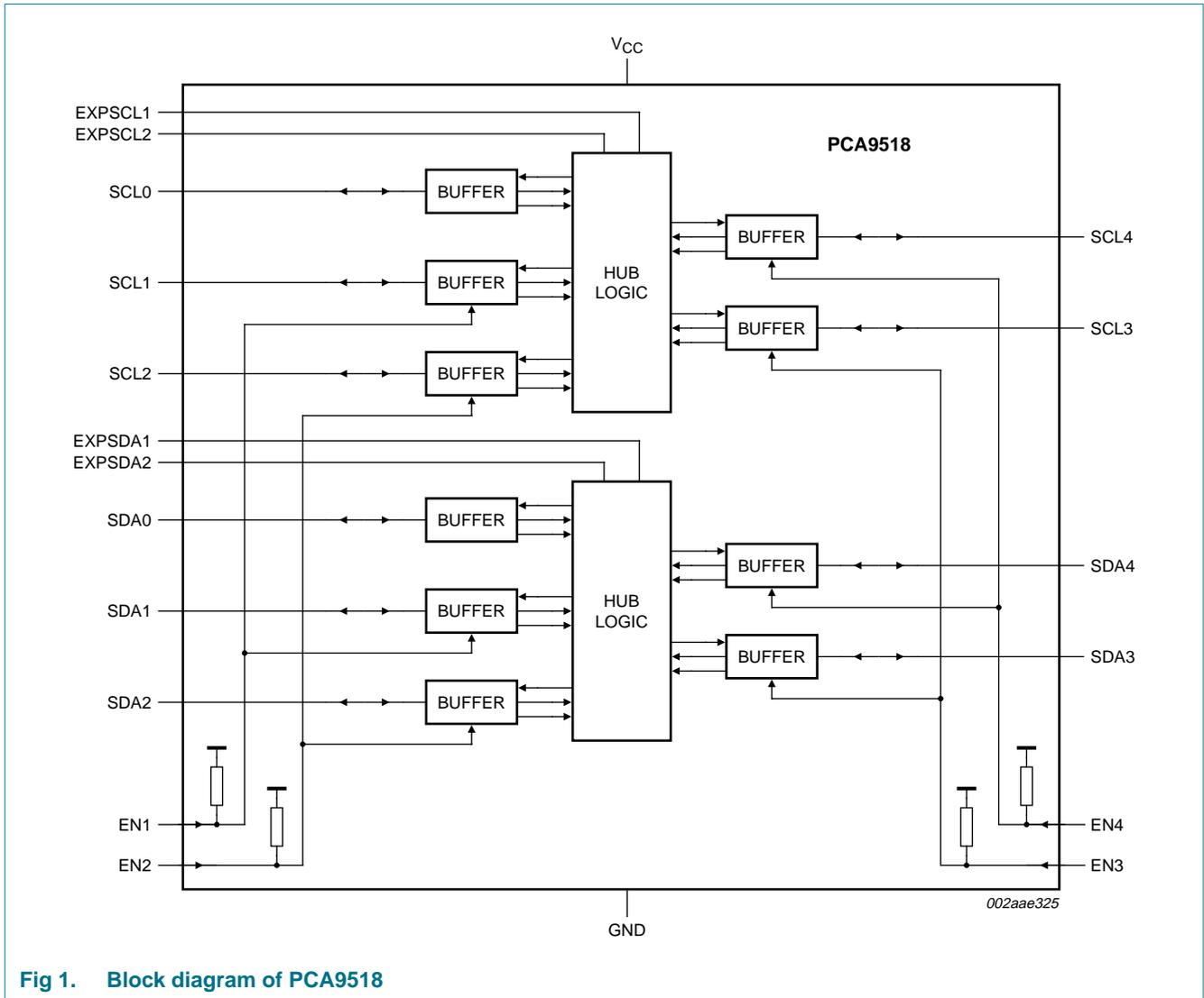
Fig 1. Block diagram of PCA9518
