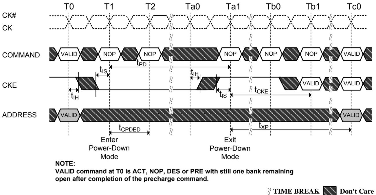
**Figure 56. Power-Down Entry after Read and Read with Auto Precharge**
