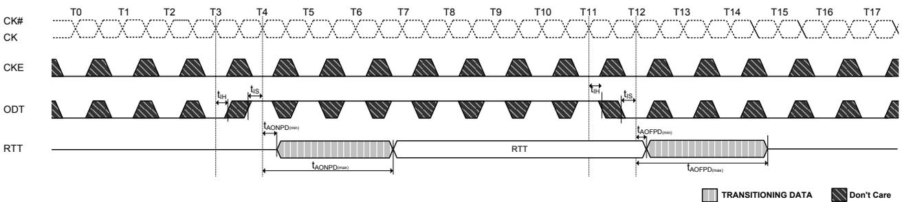
**Figure 73. Synchronous to asynchronous transition during Precharge Power Down**
