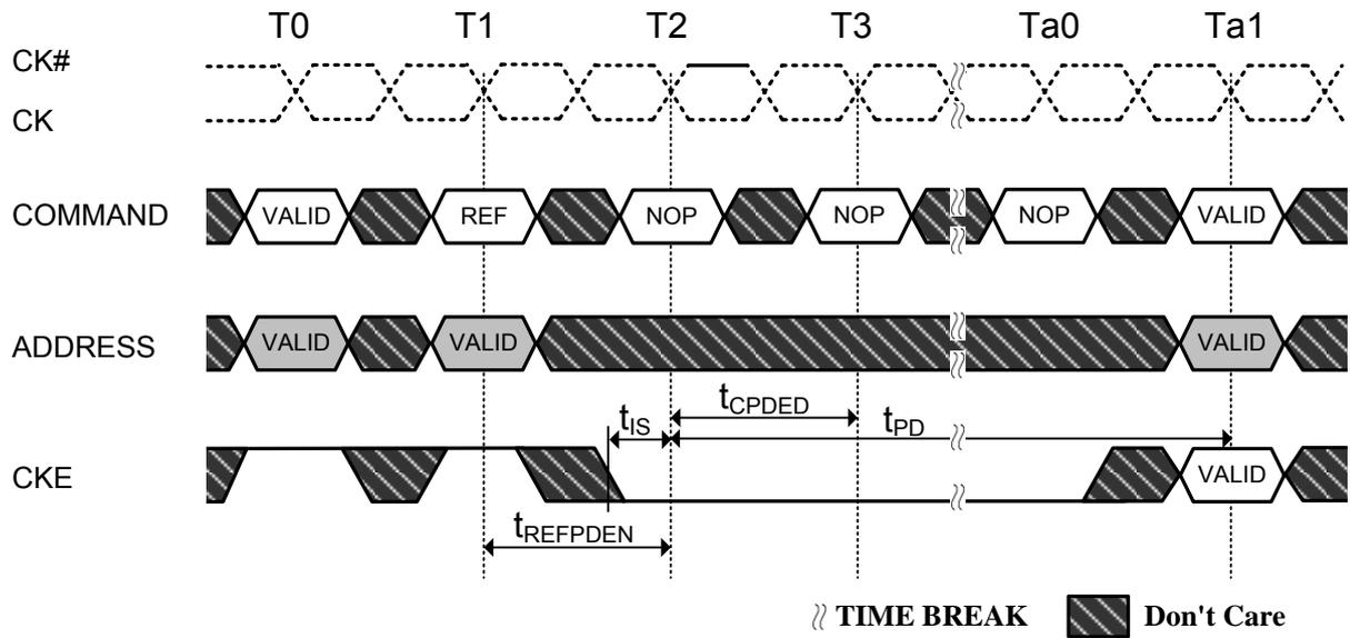
**Figure 62. Active Command to Power-Down Entry**
