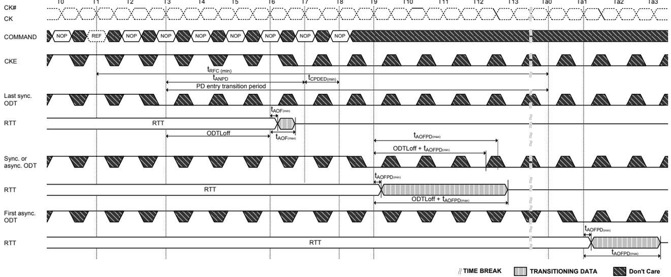
**Figure 74. Synchronous to asynchronous transition after Refresh command**
