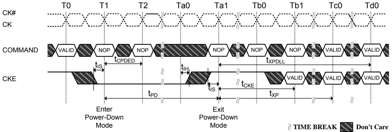
**Figure 61. Refresh Command to Power-Down Entry**
