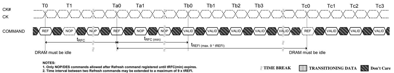
**Figure 54. Self-Refresh Entry/Exit Timing**
