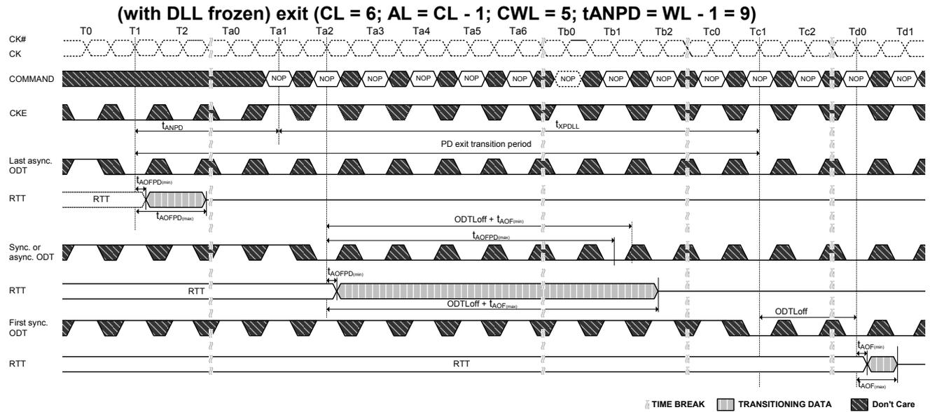
**Figure 76. Transition period for short CKE cycles, entry and exit period overlapping**
