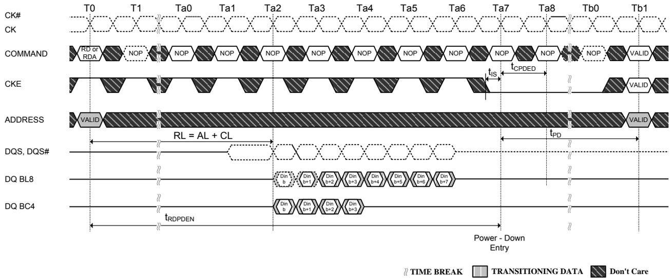
**Figure 57. Power-Down Entry after Write with Auto Precharge**
