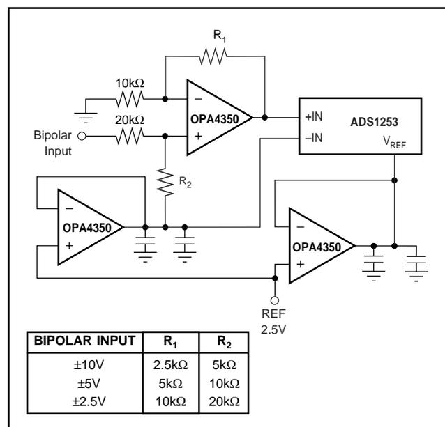
FIGURE 1. Level-Shift Circuit for Bipolar Input Ranges.
