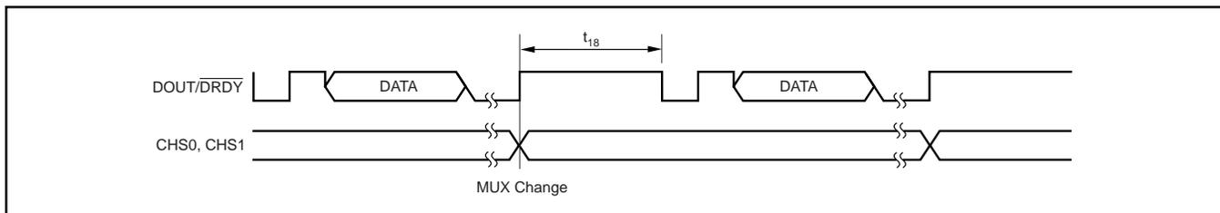
FIGURE 12. Multiplexer Operation.
