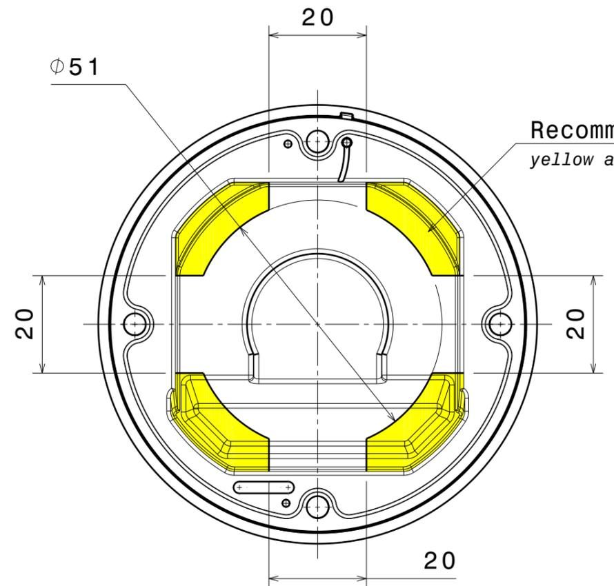
Recommended inlet area for wiring
