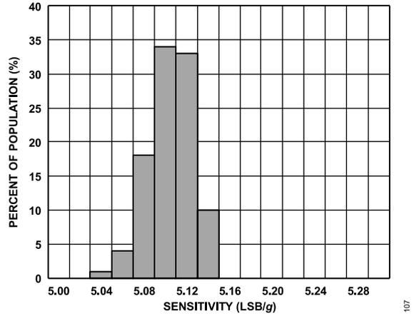
Figure 16. X-Axis Sensitivity at 25°C, V<sub>S</sub> = 2.1 V
