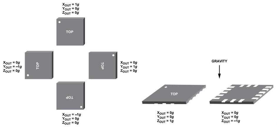
Figure 58. Output Response vs. Orientation to Gravity
