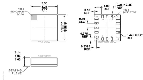
Figure 61. 16-Terminal Land Grid Array [LGA] (CC-16-4)
