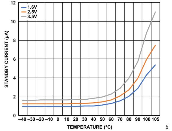
Figure 40. Standby Current vs. Temperature, Instant On Mode
