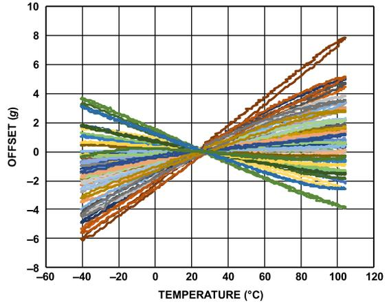
Figure 22. X-Axis 0 g Normalized Offset vs. Temperature
