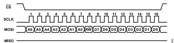
**Figure 4. SPI Timing Diagram, Single Byte Write**
