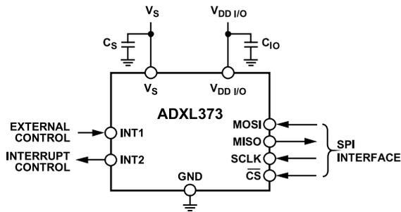
Figure 54. INT1 Pin as Input for External Clock
