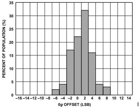
Figure 14. Y-Axis 0 g Offset at 25°C, V<sub>S</sub> = 2.1 V
