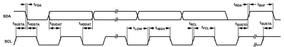
Figure 7. I<sup>2</sup>C Timing Diagram
