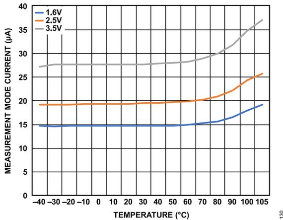
Figure 39. Measurement Mode Current vs. Temperature, Normal Mode
