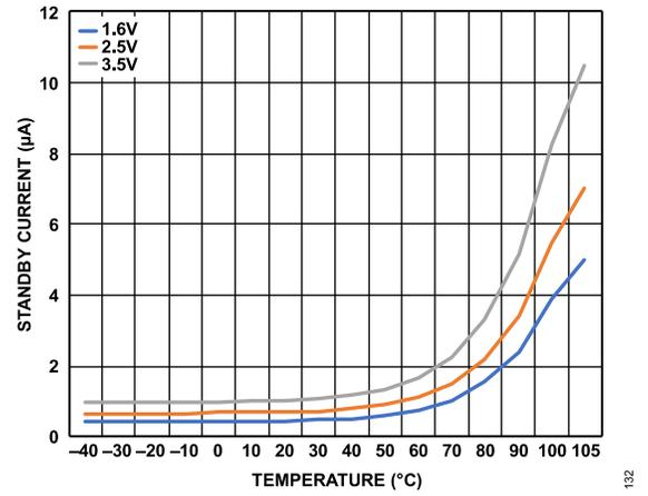
Figure 41. Standby Current vs. Temperature, Wake-Up Mode
