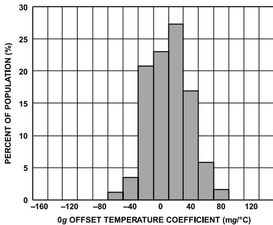
Figure 21. Z-Axis 0 g Offset Temperature Coefficient
