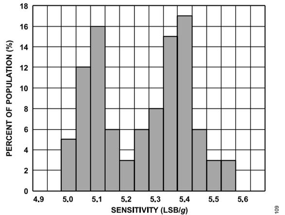
Figure 18. Z-Axis Sensitivity at 25°C, V<sub>S</sub> = 2.1 V
