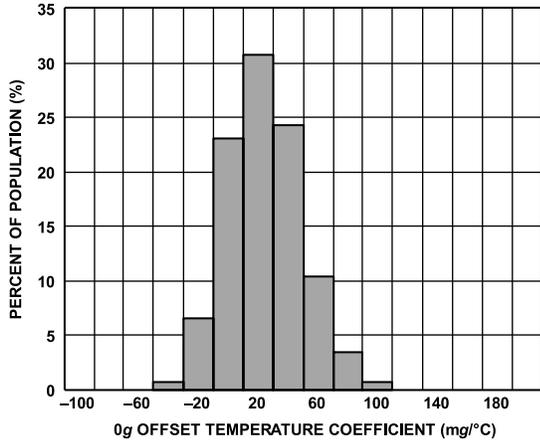
Figure 19. X-Axis 0 g Offset Temperature Coefficient
