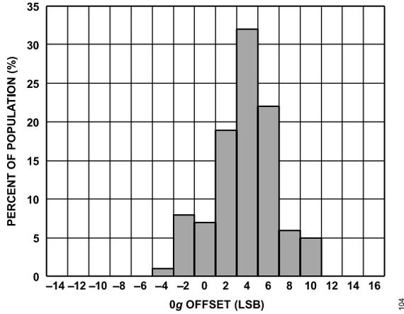
Figure 13. X-Axis 0 g Offset at 25°C, V<sub>S</sub> = 2.1 V
