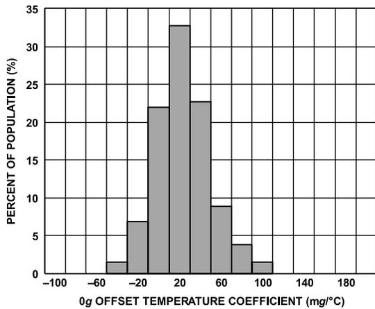
Figure 20. Y-Axis 0 g Offset Temperature Coefficient
