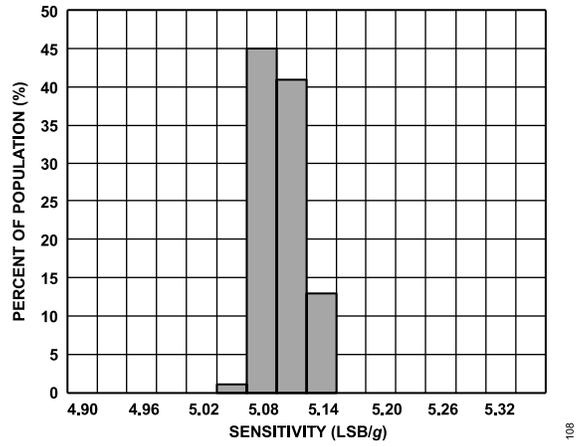
Figure 17. Y-Axis Sensitivity at 25°C, V<sub>S</sub> = 2.1 V
