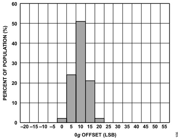
Figure 15. Z-Axis 0 g Offset at 25°C, V<sub>S</sub> = 2.1 V
