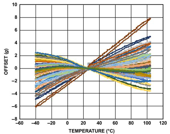
Figure 24. Z-Axis 0 g Normalized Offset vs. Temperature
