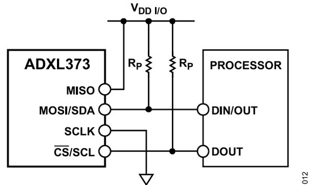
Figure 51. I<sup>2</sup>C Connection Diagram (Address 0x53)
