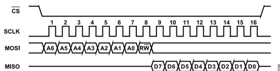
**Figure 3. SPI Timing Diagram, Single Byte Read**
