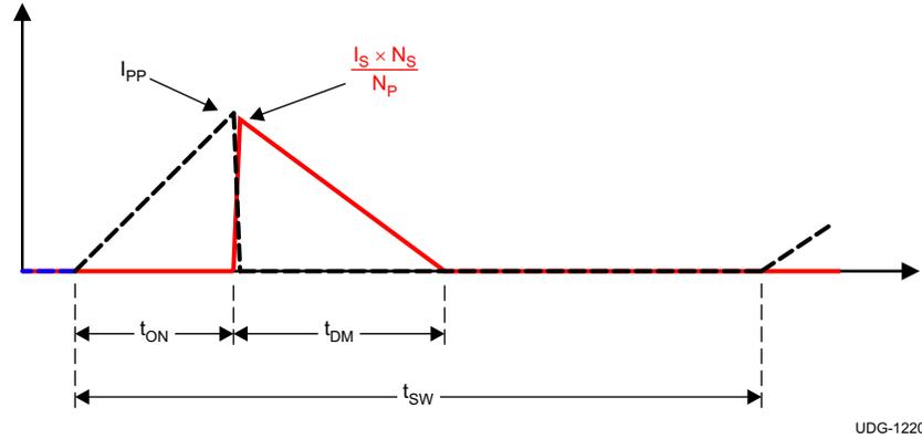
Figure 7-6. Transformer-Current Relationship
