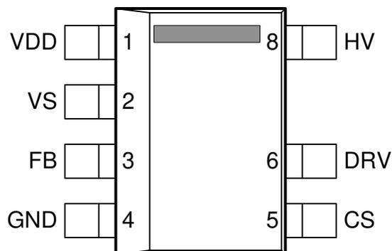
Figure 5-1. D Package 7-Pin SOIC Top View
