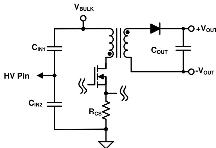
Figure 8-1. Implementation to Support > 700 V Inputs
