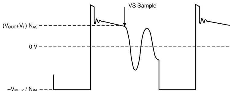
**Figure 7-3. Auxiliary-Winding Voltage**
