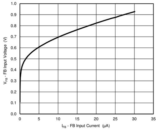
**Figure 6-9. FB Input Voltage vs. FB Input Current**
