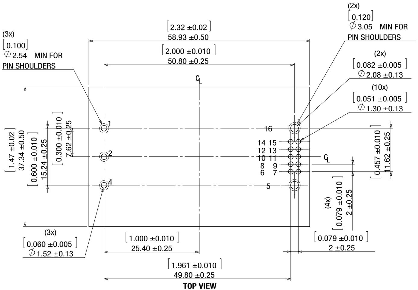
**MECHANICAL SPECIFICATIONS (NO PMBUS) WITH HEAT SINK**
