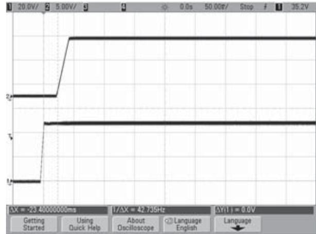
Stepload Transient Response (Vin = 48V, Iout = 50-75-50% of Iout, Load = 1000μF)
