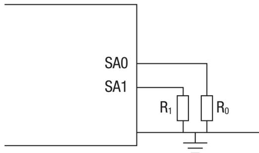
Figure 2. Schematic of Connection of Address Resistors
