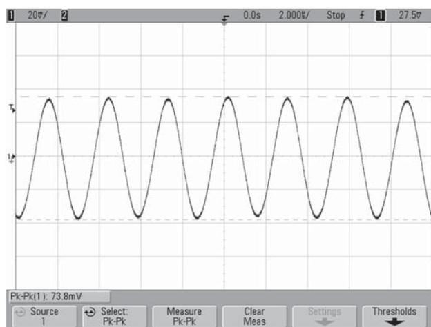
Output Ripple & Noise (Vin = 48V, Iout = 50A, Cout = 1μF || 10μF, Ta = +25°C)
