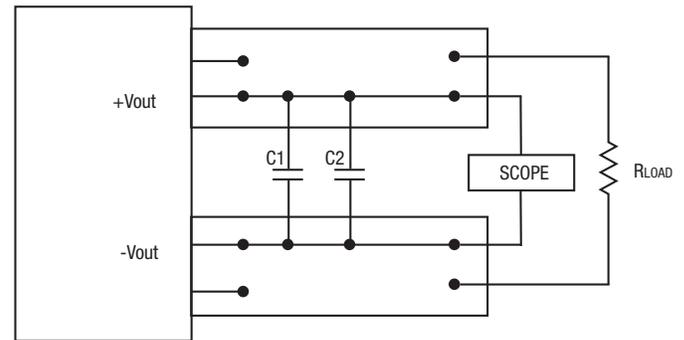
$C1 = 1\mu\text{F}$ ;  $C2 = 10\mu\text{F}$
