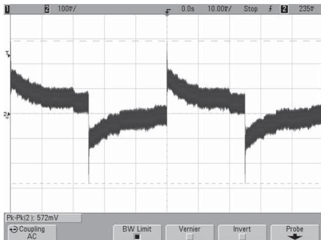
Stepload Transient Response (Vin = 48V, Iout = 25-75-25% of Iout, Load = 1000μF)
