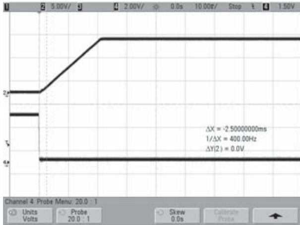
Startup Delay (Vin = 48V, Iout = 50A, Cout = 10000μF, Ta = +25°C)
