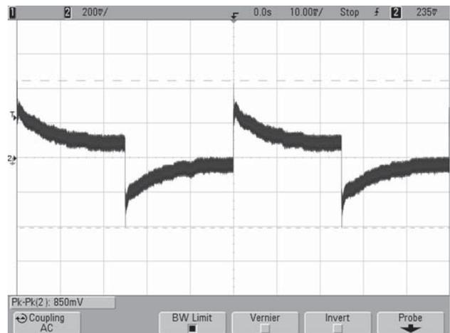
Output Ripple & Noise (Vin = 48V, Iout = 0A, Cout = 1μF || 10μF, Ta = +25°C)
