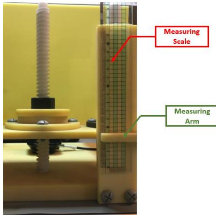
The test sample is placed on a thin sheet of plastic connected to the moveable part of the fixture. Then the distance is carefully adjusted until the reader can no longer read the sample, thus the maximum interrogation distance is displayed in the ruler.
