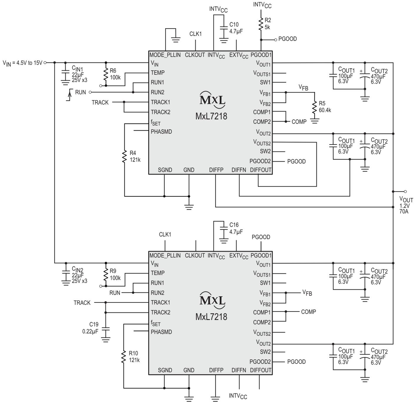
**Figure 18: MxL7218 2-Module, 4-Phase, 1.2V, 70A Regulator**
