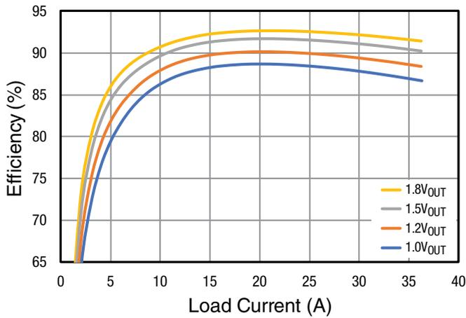
**Figure 6: Efficiency: Dual Phase,  $V_{IN} = 12V$ , 450kHz**
