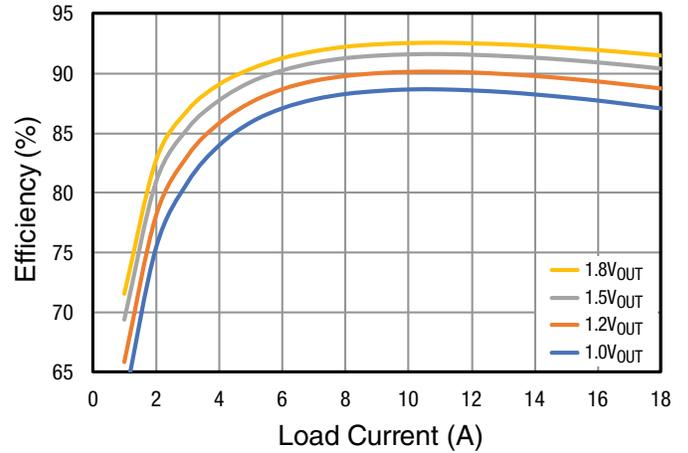
**Figure 5: Efficiency: Single Phase,  $V_{IN} = 12V$ , 450kHz**
