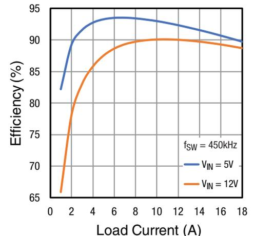
**Figure 2:** 1.2V<sub>OUT</sub> Efficiency vs I<sub>OUT</sub>
