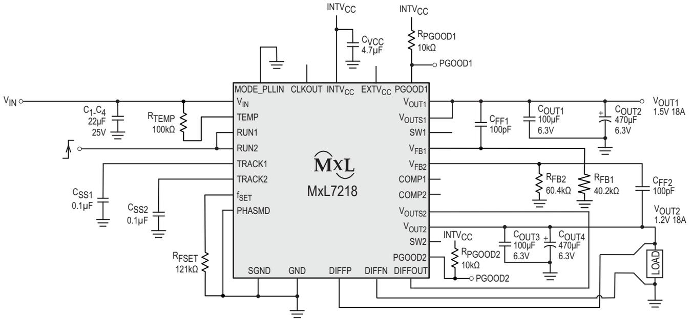
**Figure 17: Typical 4.5V<sub>IN</sub> to 15V<sub>IN</sub>, 1.5V and 1.2V at 18A Outputs**
