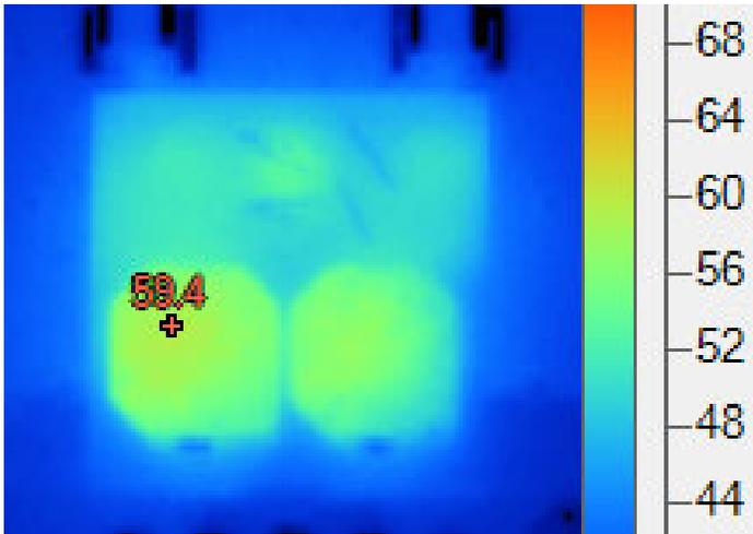
**Figure 31:** Thermal Image 12V to 1V, 36A with 200LFM<sup>(1)</sup>
