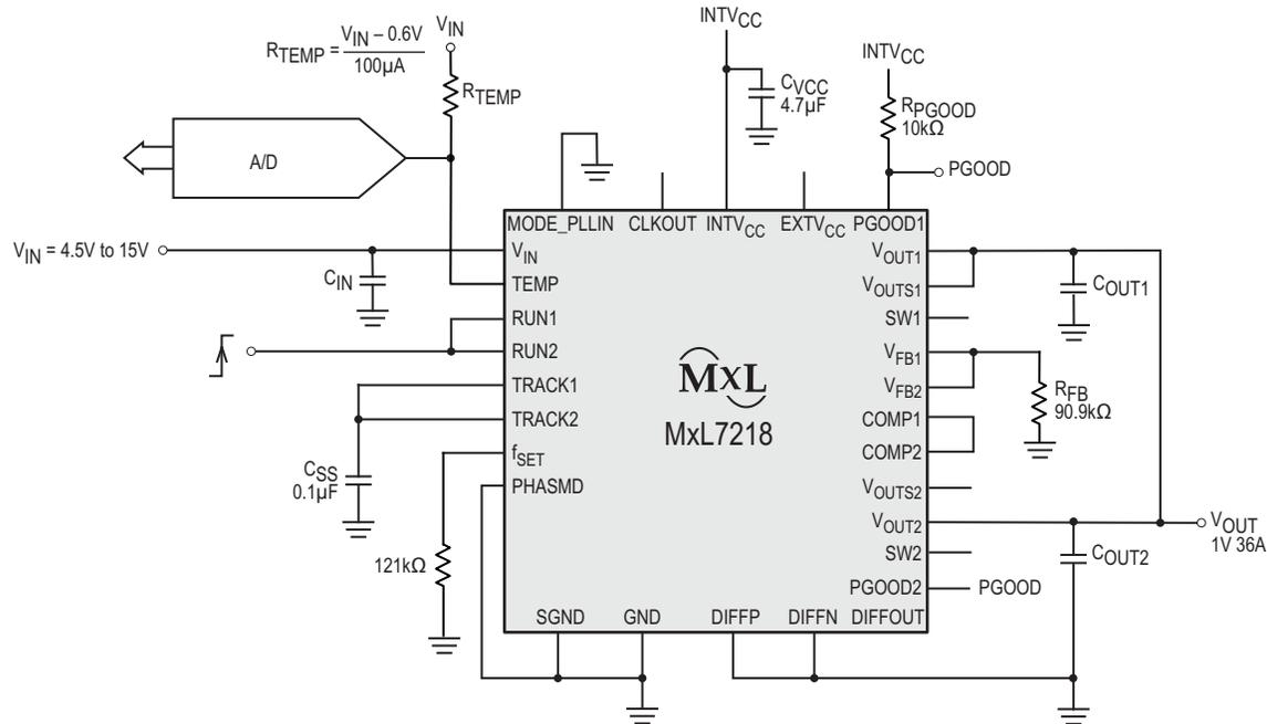
**Figure 30: 2-Phase, 1V at 36A with Temperature Monitoring**
