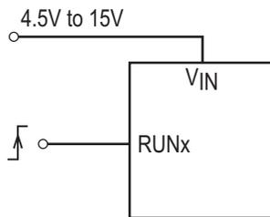
**Figure 26: RUNx Pin Driven by a Logic Signal**
