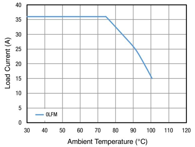
**Figure 38: 12V to 1V Current Derating**
