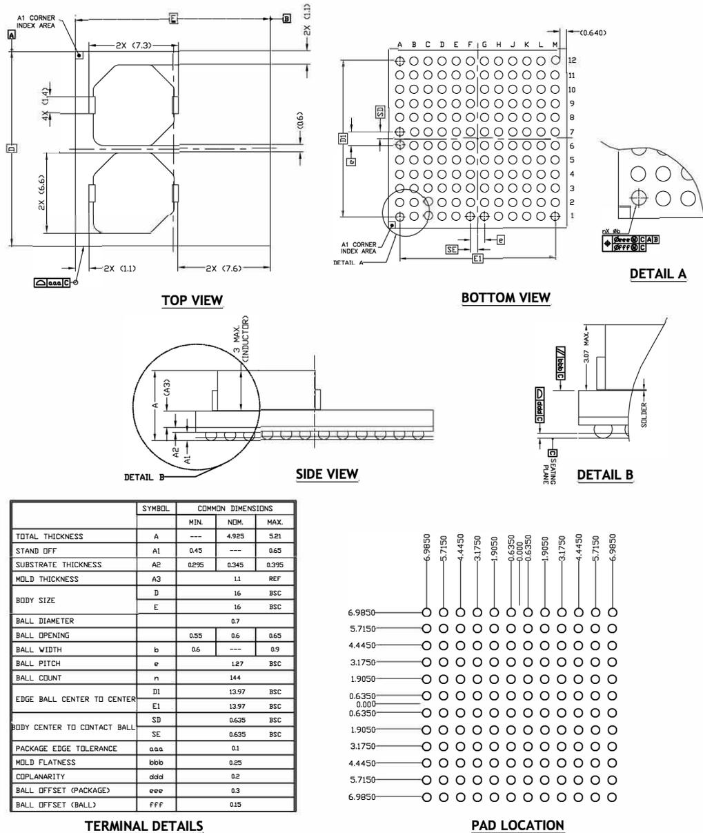
NOTE : ALL DIMENSIONS ARE IN MILLIMETERS, ANGLES ARE IN DEGREES.
