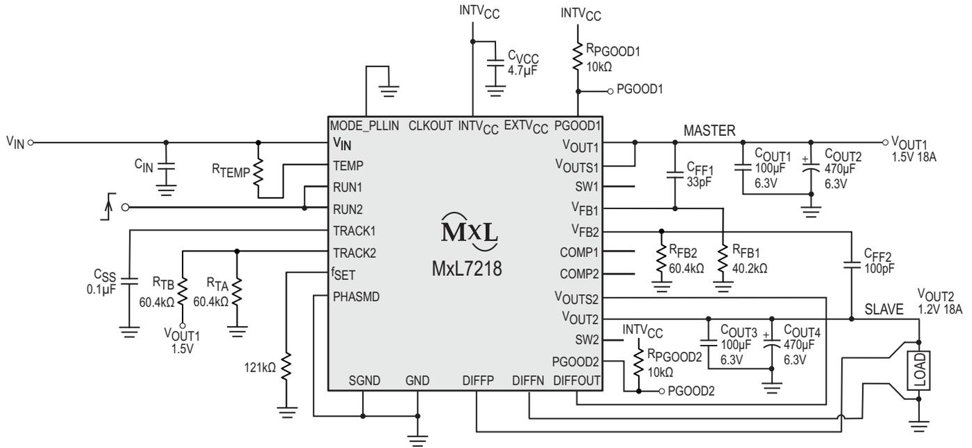
**Figure 24: Example of Output Tracking Application Circuit**
