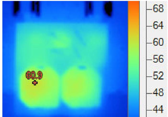
**Figure 32:** Thermal Image 12V to 1.2V, 36A with 200LFM<sup>(1)</sup>
