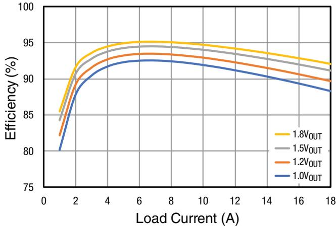
**Figure 4: Efficiency: Single Phase,  $V_{IN} = 5V$ , 450kHz**
