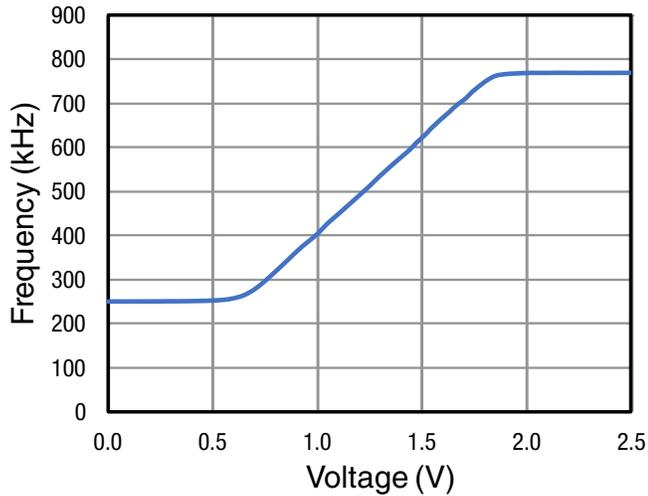
**Figure 22:** Operating Frequency vs.  $f_{SET}$  Pin Voltage
