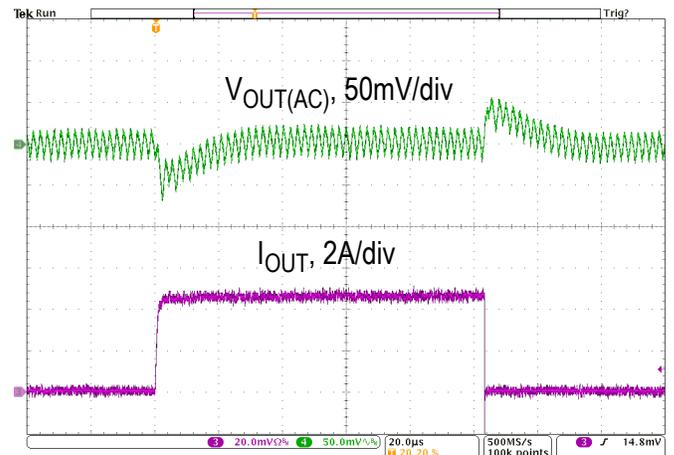
$C_{OUT} = 1 \times 470\mu\text{F } 4\text{V POSCAP} + 1 \times 100\mu\text{F } 6.3\text{V Ceramic}$
