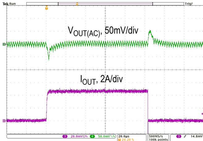
$C_{OUT} = 1 \times 470\mu\text{F } 4\text{V POSCAP} + 1 \times 100\mu\text{F } 6.3\text{V Ceramic}$
