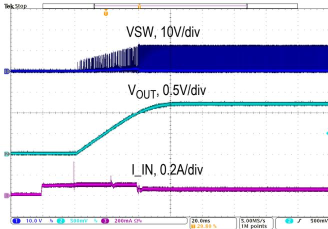
$C_{OUT} = 1 \times 470\mu\text{F POSCAP} + 1 \times 100\mu\text{F Ceramic}$
