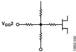
Figure 4. V<sub>GG2</sub> Interface Schematic
