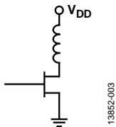
Figure 5. V<sub>DD</sub> Interface Schematic
