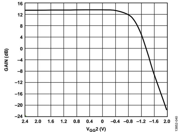
Figure 30. Gain vs.  $V_{GG2}$  at 10 GHz
