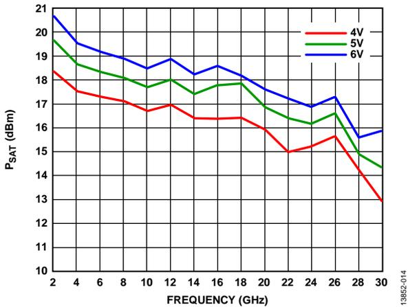
Figure 15.  $P_{SAT}$  vs. Frequency at Various Supply Voltages
