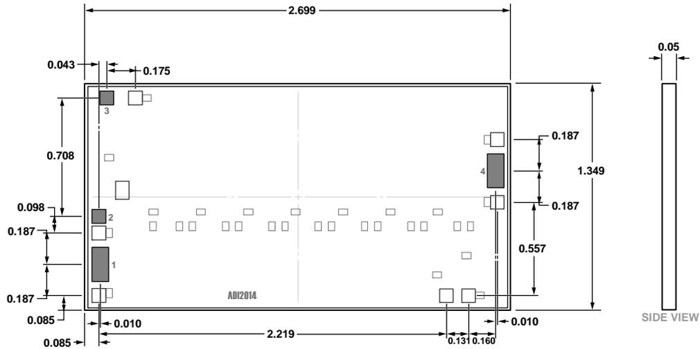
Figure 38. 4-Pad Bare Die [CHIP]
