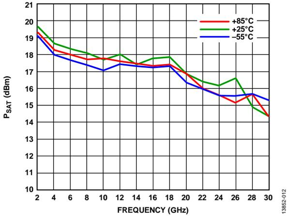
Figure 14.  $P_{SAT}$  vs. Frequency at Various Temperatures
