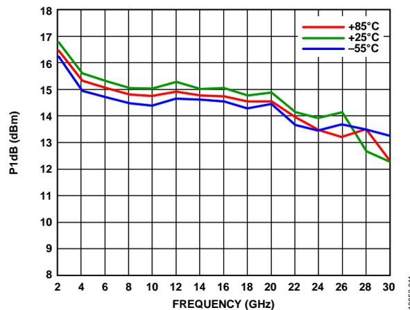
Figure 13. P1dB vs. Frequency at Various Temperatures
