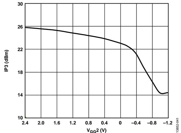
Figure 31. Output IP3 vs.  $V_{GG2}$  at 10 GHz
