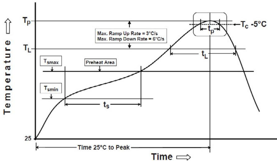
Figure 12. Solder Profile for the GNSSCP-SM12L1 Antenna
