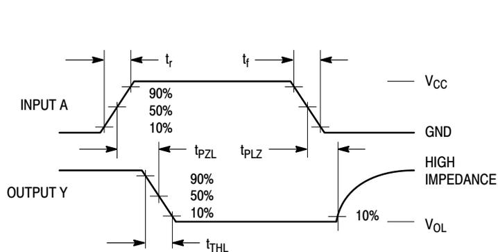
Figure 1. Switching Waveforms
