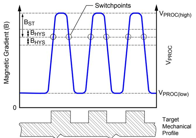
Figure 4. Running Mode Switch Point and Internal Hysteresis
