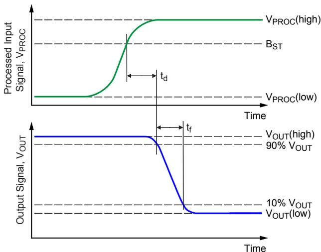
Figure 3. Output Delay Time and Output Fall Time
