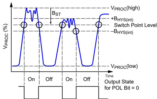
Figure 7. Switching on internal hysteresis
