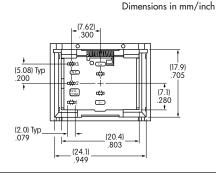
**BASE SWITCH FULL FACE ILLUMINATED CAP** AT4118 Diffuser AT4117 Lens Color: Clear Color: White Part Number UB16NKW015F-JB (15.35)
