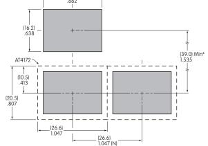
\* Minimum dimension allows opening of cover to 180° (N) = Number of switches
