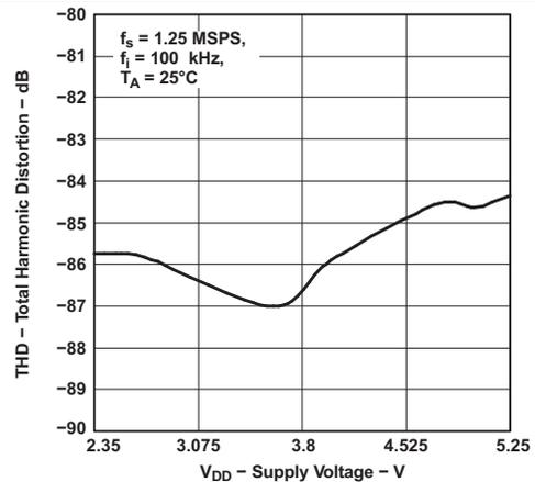
Figure 8. Total Harmonic Distortion vs Supply Voltage
