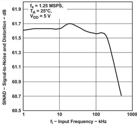
Figure 5. Signal-to-Noise and Distortion vs Input Frequency
