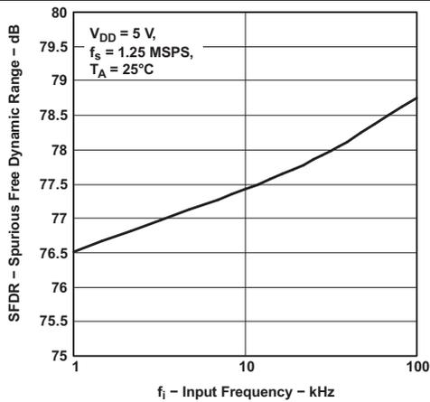
Figure 22. Spurious Free Dynamic Range vs Input Frequency
