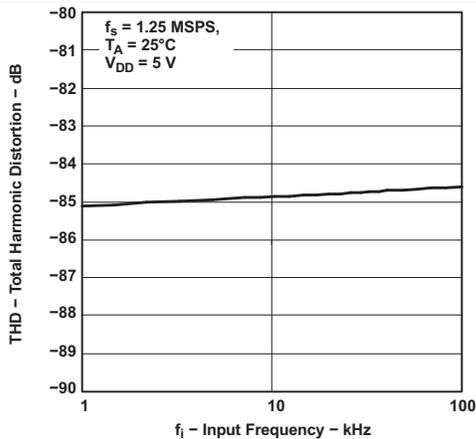
Figure 7. Total Harmonic Distortion vs Input Frequency
