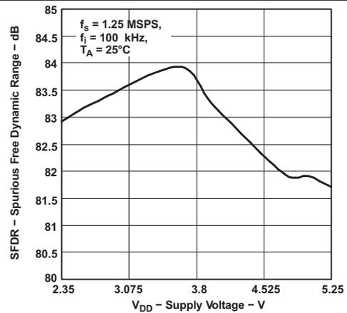
Figure 10. Spurious Free Dynamic Range vs Supply Voltage
