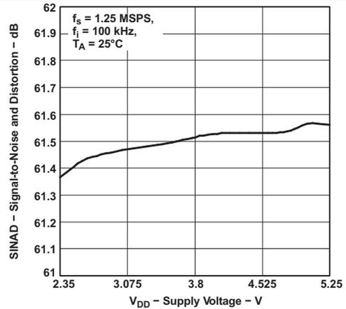
Figure 6. Signal-to-Noise and Distortion vs Supply Voltage
