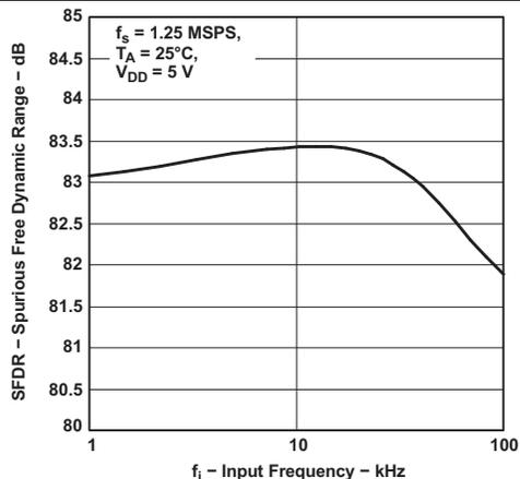
Figure 9. Spurious Free Dynamic Range vs Input Frequency
