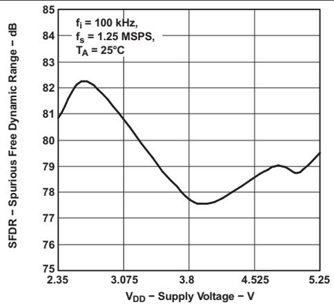
Figure 23. Spurious Free Dynamic Range vs Supply Voltage
