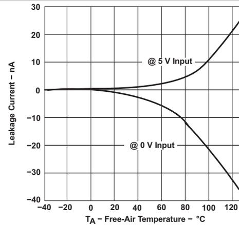
Figure 4. Analog Input Leakage Current vs Free-Air Temperature
