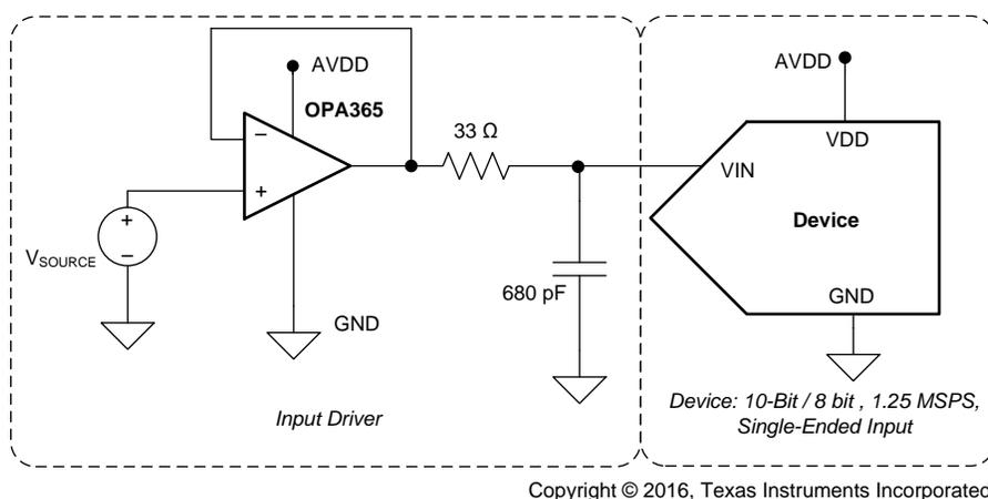
**Figure 37. Typical Data Acquisition (DAQ) Circuit: Single-Supply DAQ**
