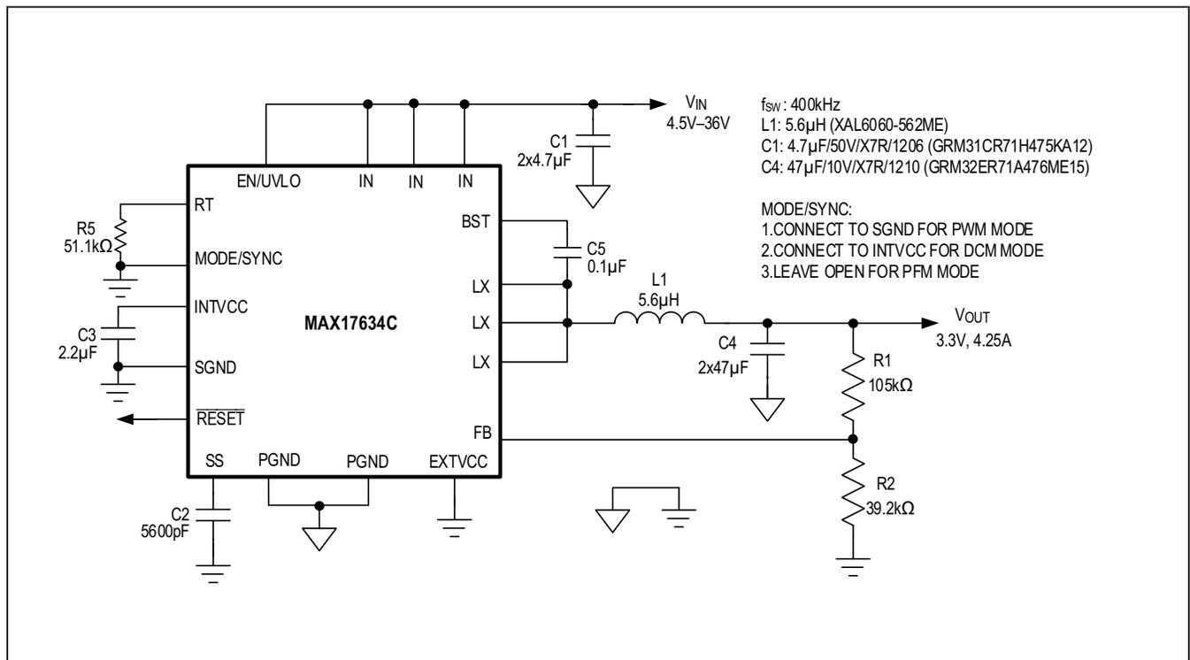
Figure 3. Adjustable 3.3V Output with 400kHz Switching Frequency
