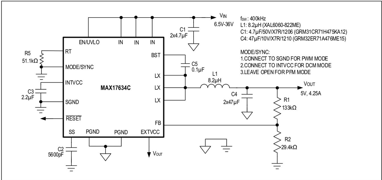
Figure 4. Adjustable 5V Output with 400kHz Switching Frequency
