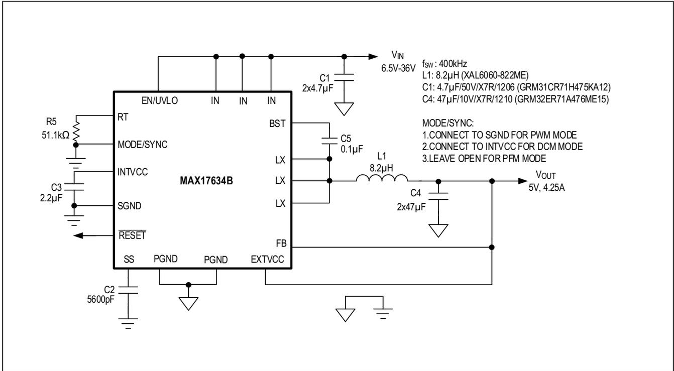
Figure 6. Fixed 5V Output with 400kHz Switching Frequency
