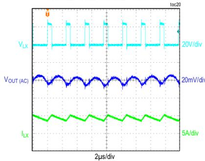
CONDITIONS: 5V OUTPUT, PWM MODE, 4.25A LOAD
