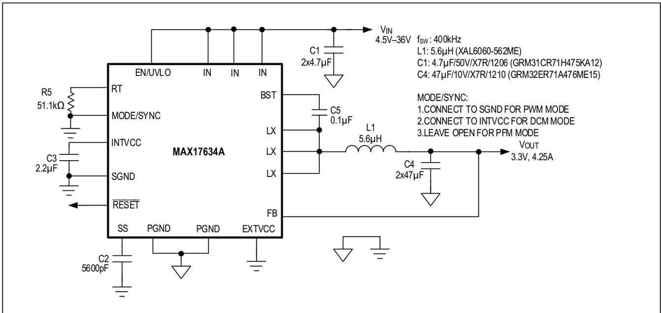
Figure 5. Fixed 3.3V Output with 400kHz Switching Frequency
