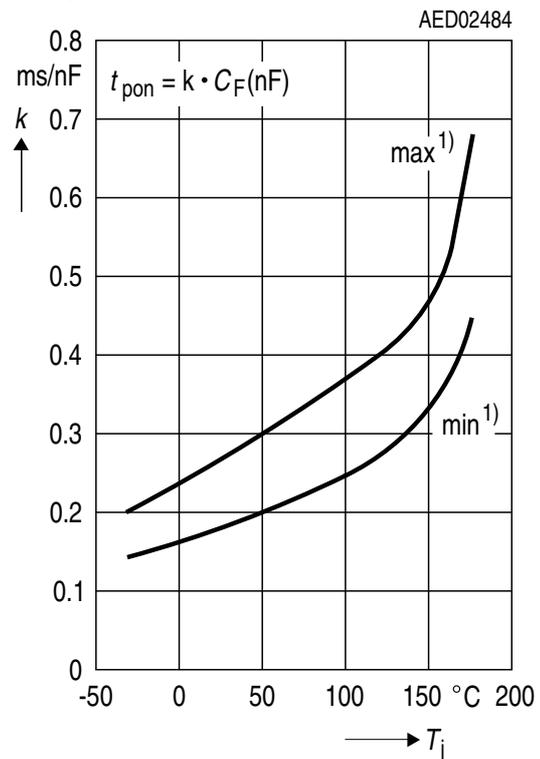
1) Calculated values for minimum and maximum filter resistance,  $C_F$  at room temperature.
