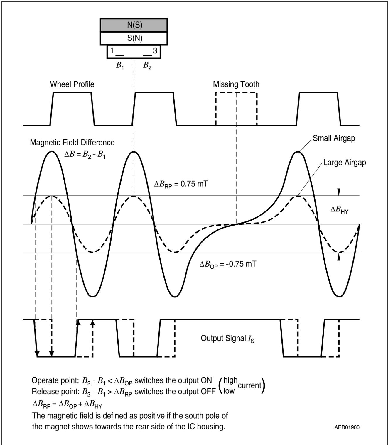
Figure 13 System Operation
