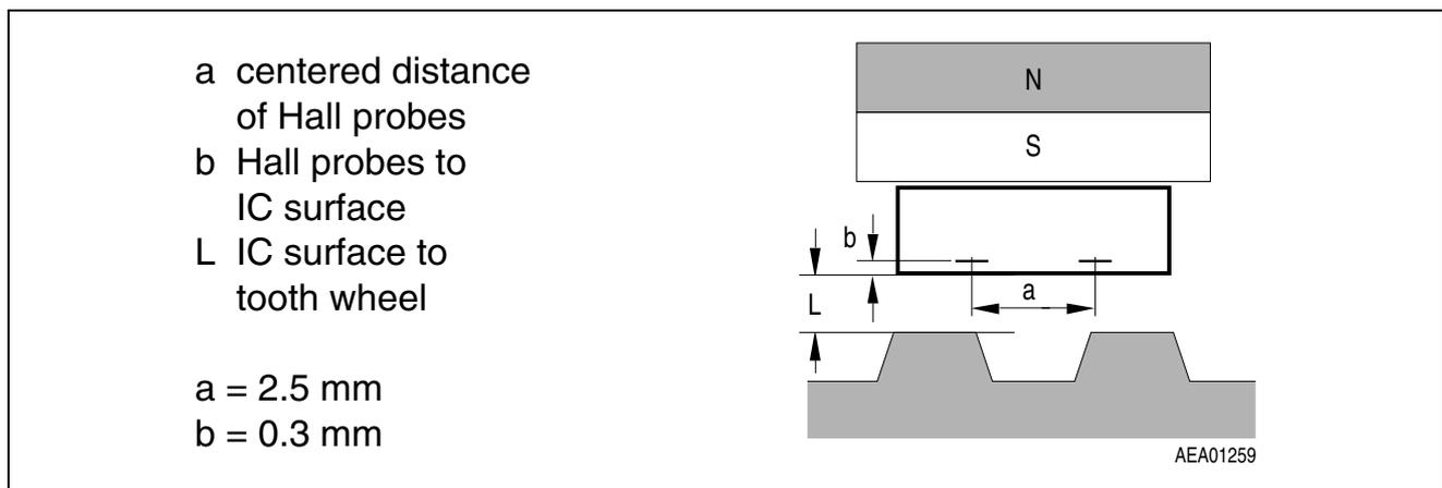
**Figure 8 Sensor Spacing**
