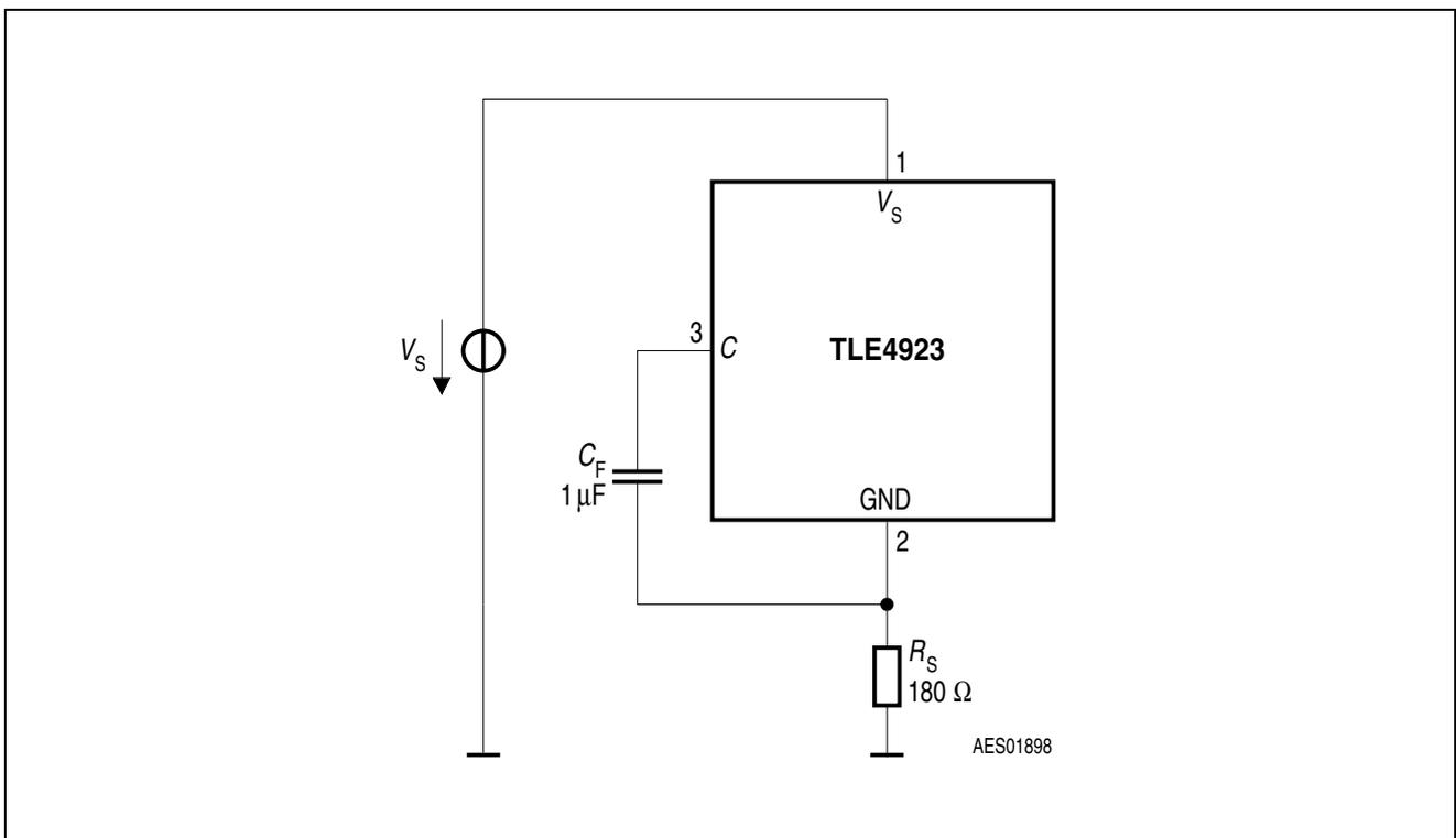
Figure 4 Test Circuit 2
