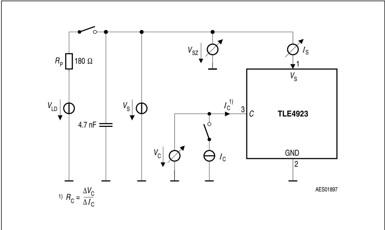
Figure 3 Test Circuit 1
