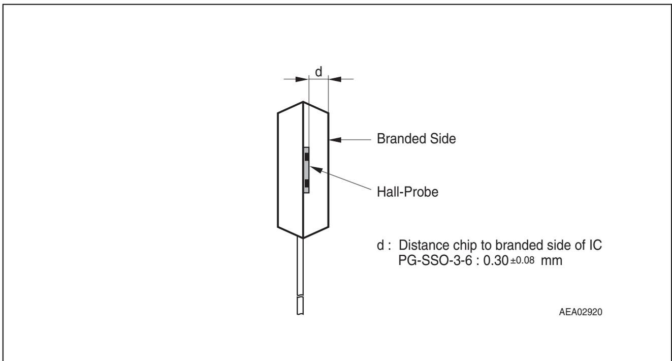
Figure 14 Distance Chip to Upper Side of IC
