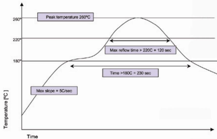
Figure 6 – High Temperature Solder Reflow Thermal Profile
