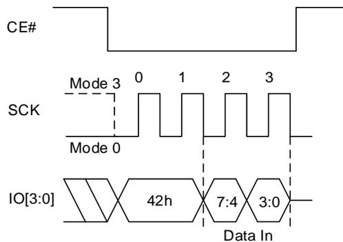
**8.22 ENTER QUAD PERIPHERAL INTERFACE (QPI) MODE OPERATION (QPIEN, 35h; QPIDI, F5h)**
