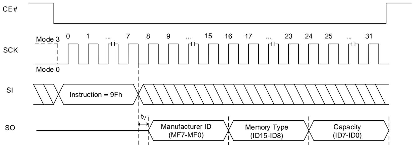
**Figure 8.50 RDJDID and RDJDIDQ (Read JEDEC ID) Sequence In QPI Mode**
