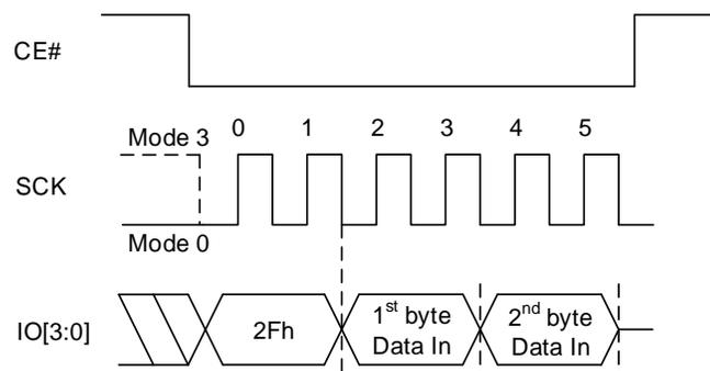
**8.54 READ PPB LOCK BIT OPERATION (RDPLB, A7h)**
