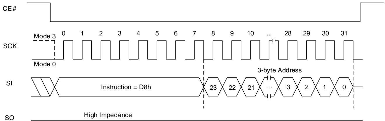
**Figure 8.16 Block Erase (64K) Sequence In QPI Mode (D8h)**
