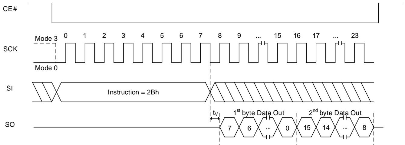
**Figure 8.85 Read ASP Sequence In QPI Mode**
