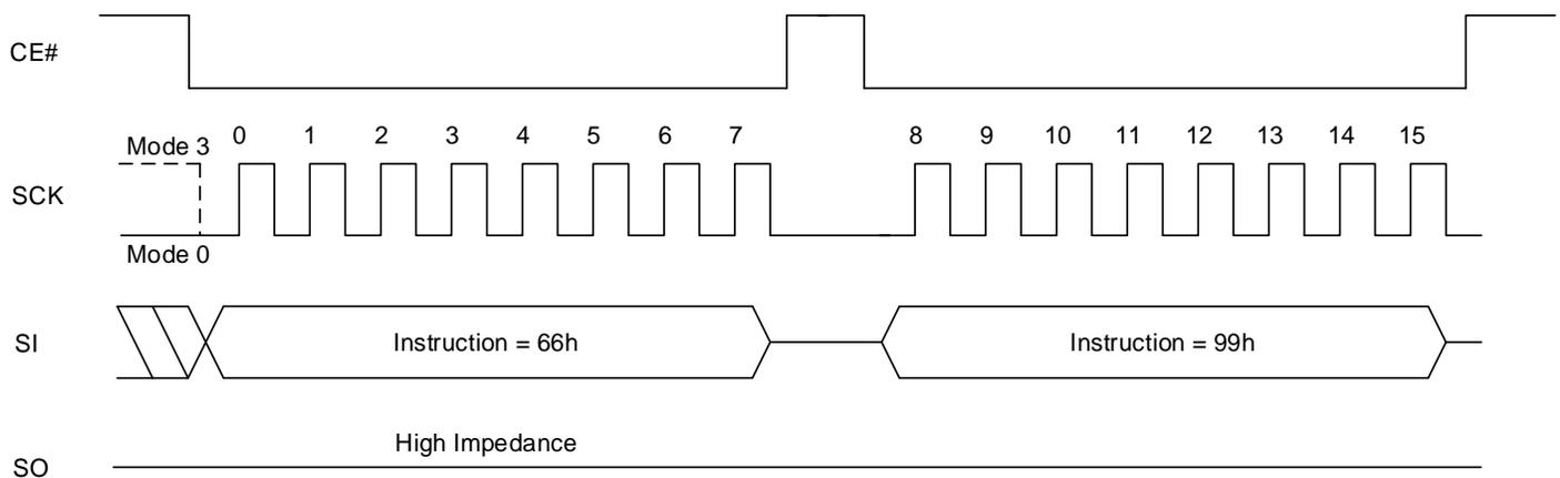
**Figure 8.56 Software Reset Enable and Software Reset QPI Sequence (RSTEN, 66h + RST, 99h)**
