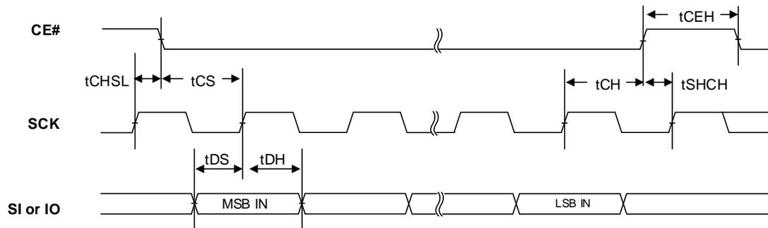
Figure 9.3 SERIAL INPUT TIMING (DTR Mode)
