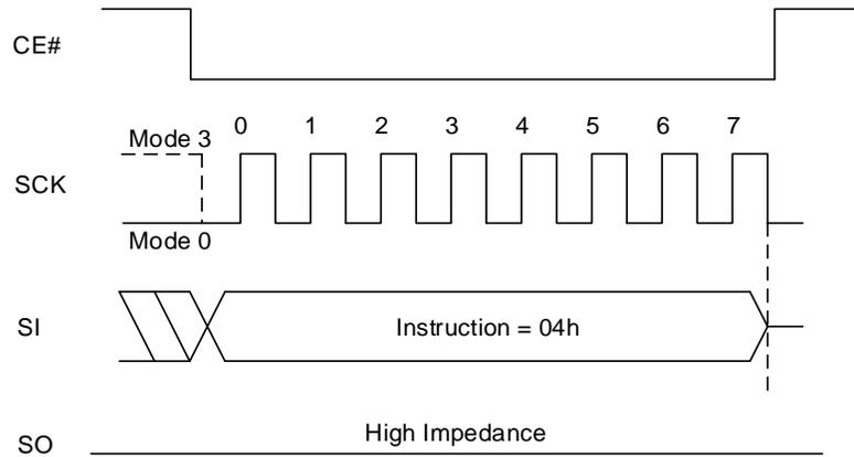
**Figure 8.22 Write Disable Sequence In QPI Mode**
