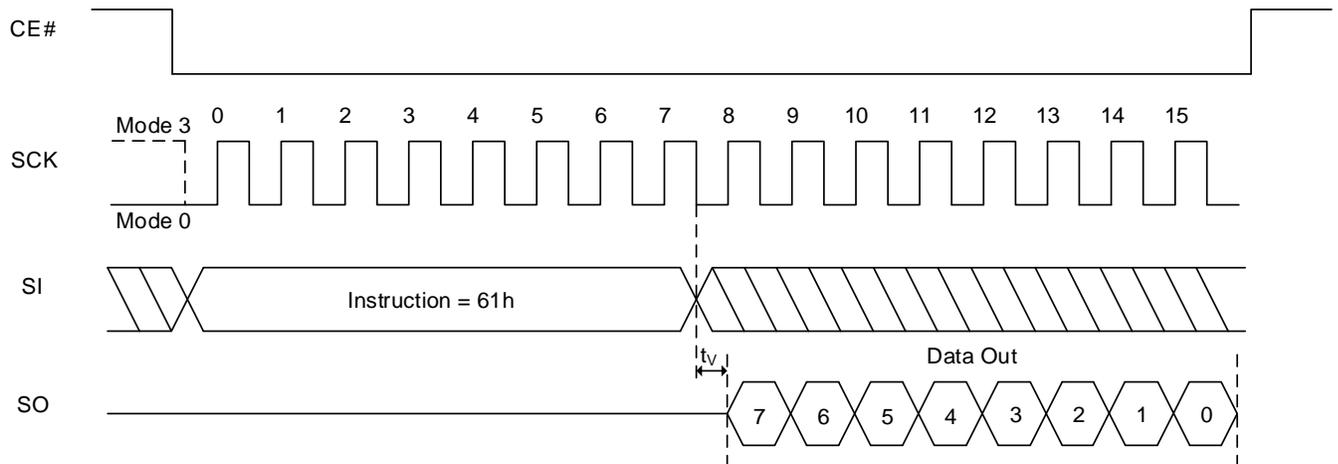
**Figure 8.42 Read Read Parameters Sequence In QPI Mode**
