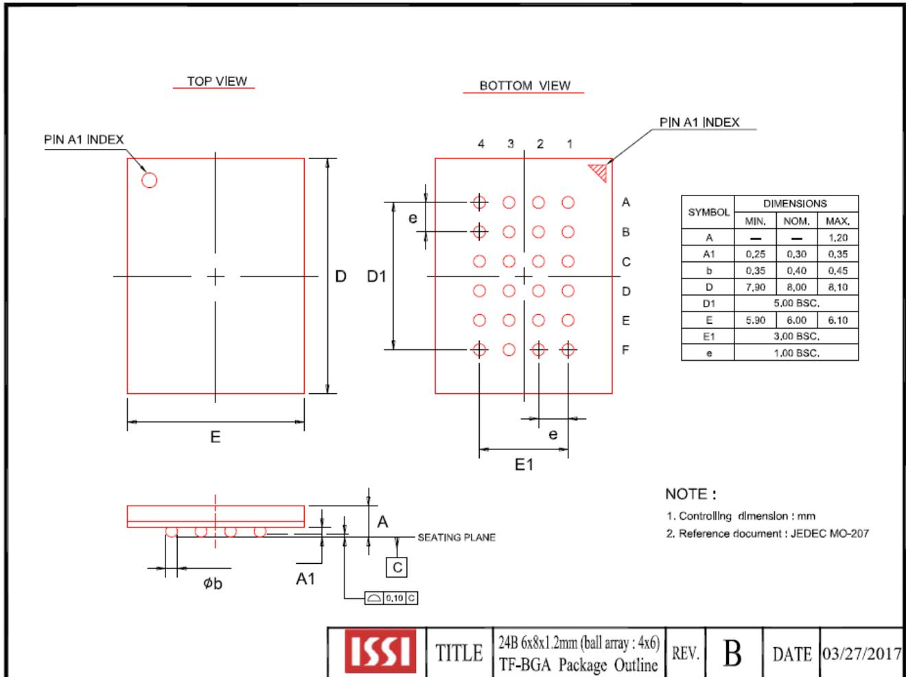
**10.5 24-BALL THIN PROFILE FINE PITCH BGA 6X8MM 5X5 BALL ARRAY (H)**
