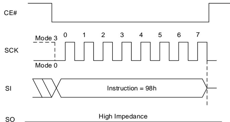
**Figure 8.101 Gang Sector/Block Unlock Sequence In QPI Mode**
