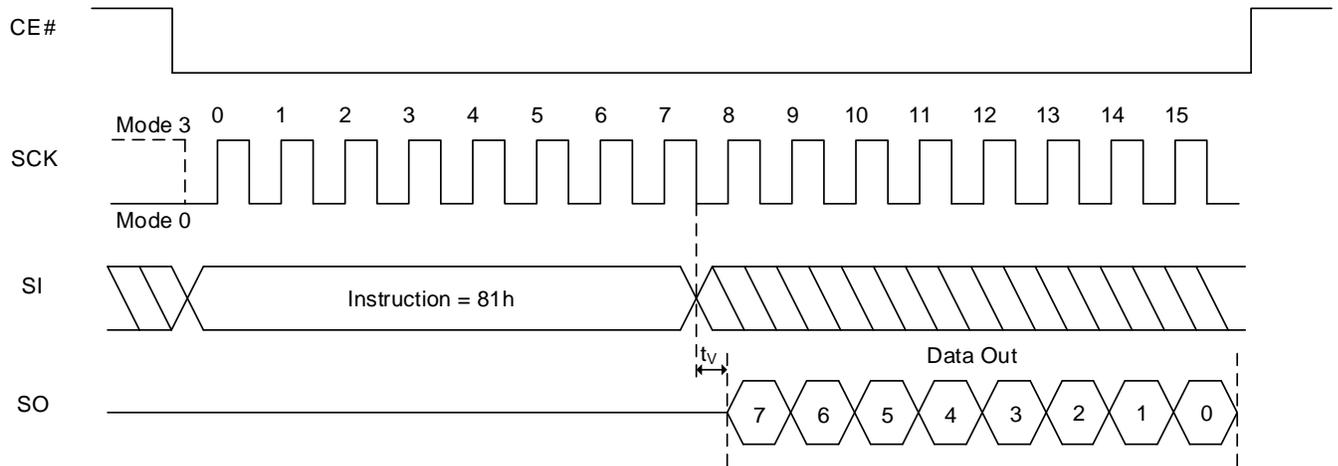
**Figure 8.44 Read Extended Read Parameters Sequence In QPI Mode**
