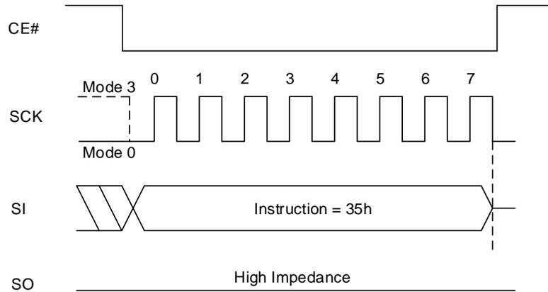
**Figure 8.32 Exit Quad Peripheral Interface (QPI) Mode Sequence**
