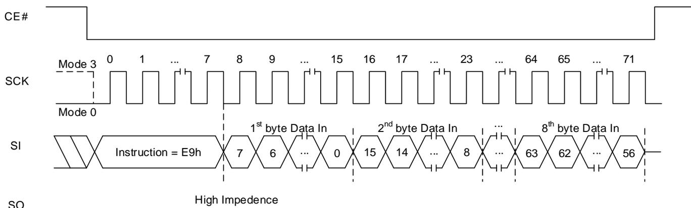
**Figure 8.97 Unlock Password Sequence In SPI Mode**
