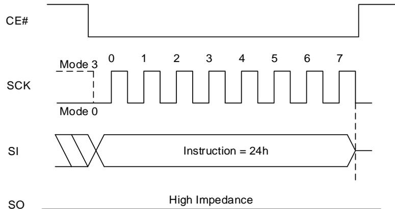
**Figure 8.69 Sector Lock Sequence In QPI Mode**
