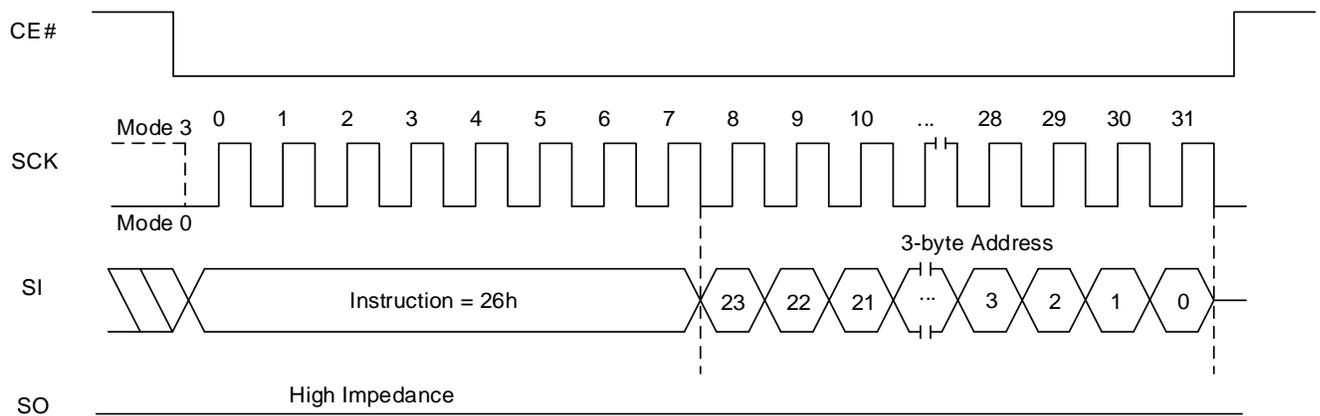
Figure 8.67 Sector Unlock Sequence In QPI Mode (26h)
