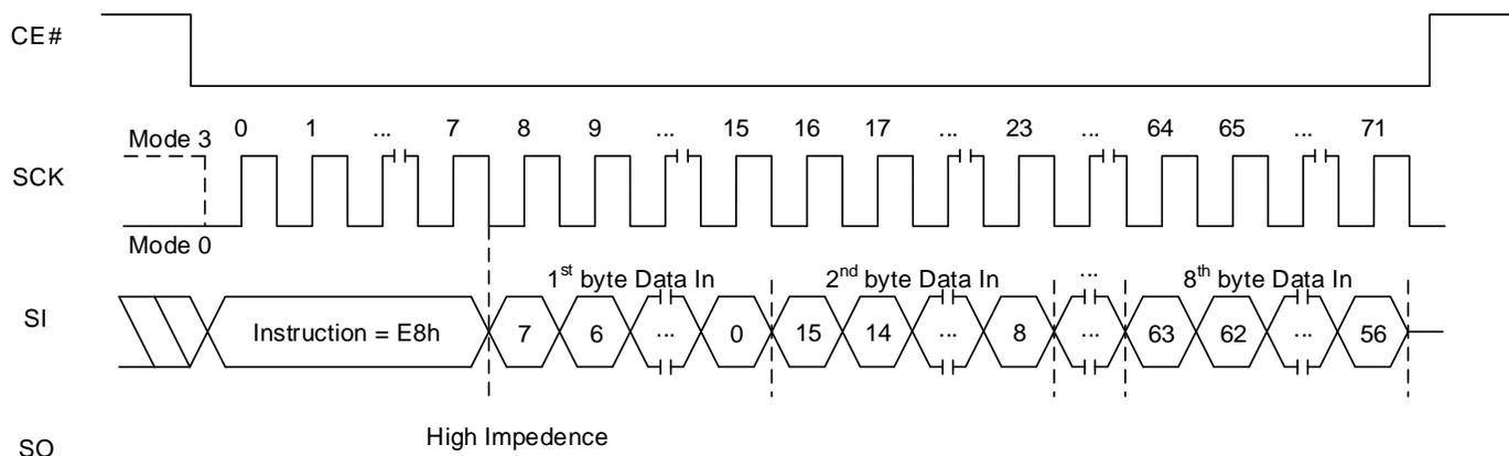
**Figure 8.95 Program Password Sequence In QPI Mode**
