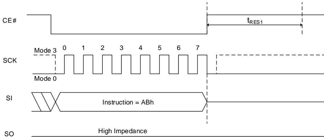
**Figure 8.36 Release Power Down Mode Sequence In QPI Mode**
