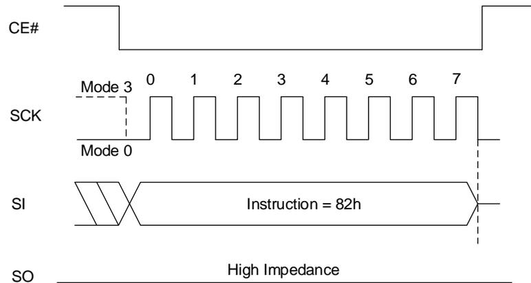
**Figure 8.46 Clear Extended Read Register Sequence In QPI Mode**
