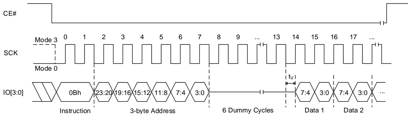
**Note: Number of dummy cycles depends on Read Parameter setting. Detailed information in Table 6.11 Read Dummy Cycles.**
