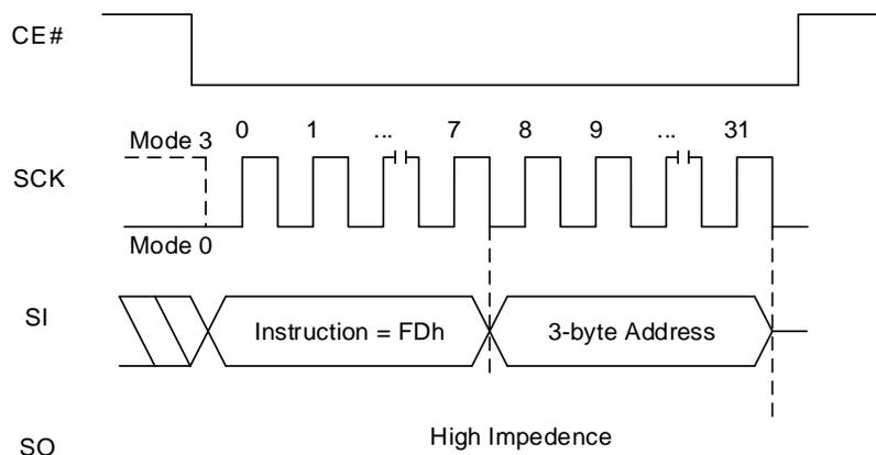
**Figure 8.81 Program PPB Sequence In QPI Mode (FDh)**
