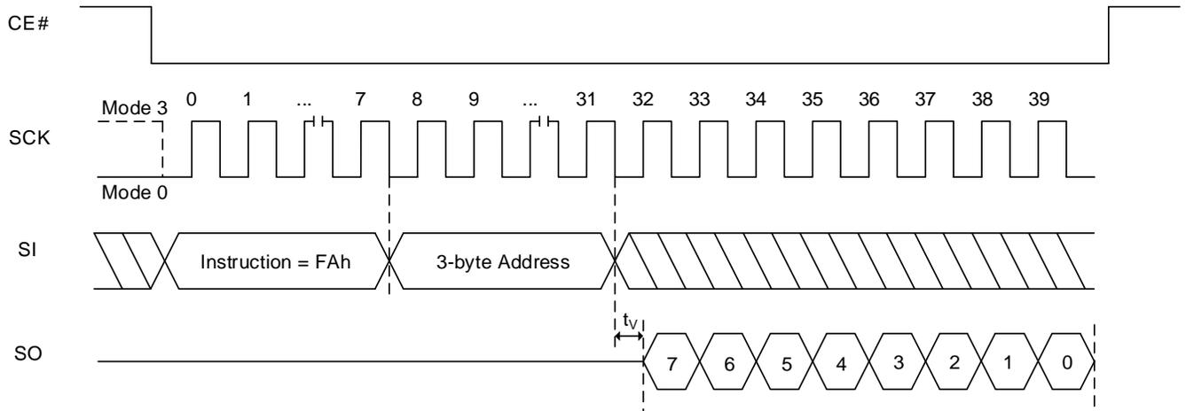
Figure 8.76 Read DYB Sequence In QPI Mode (FAh)
