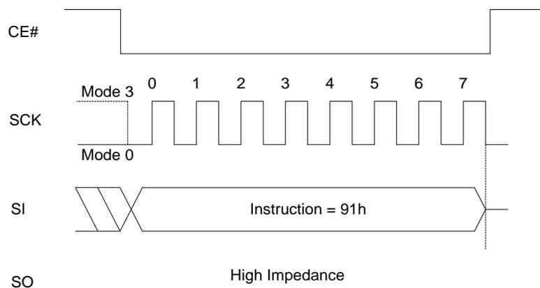
**Figure 8.92 Set FREEZE Bit Sequence In QPI Mode**
