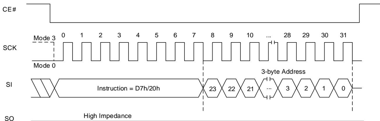
**Figure 8.14 Sector Erase Sequence In QPI Mode (D7h/20h)**
