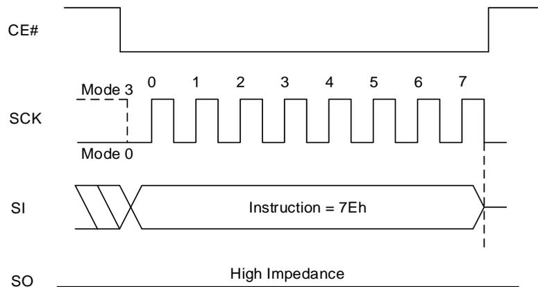
**Figure 8.99 Gang Sector/Block Lock Sequence In QPI Mode**
