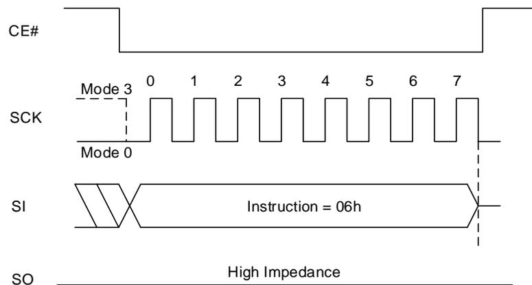
**Figure 8.20 Write Enable Sequence In QPI Mode**
