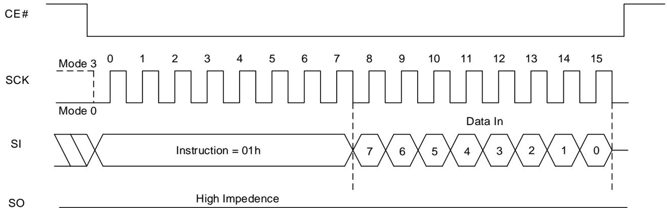
**Figure 8.26 Write Status Register Sequence In QPI Mode**
