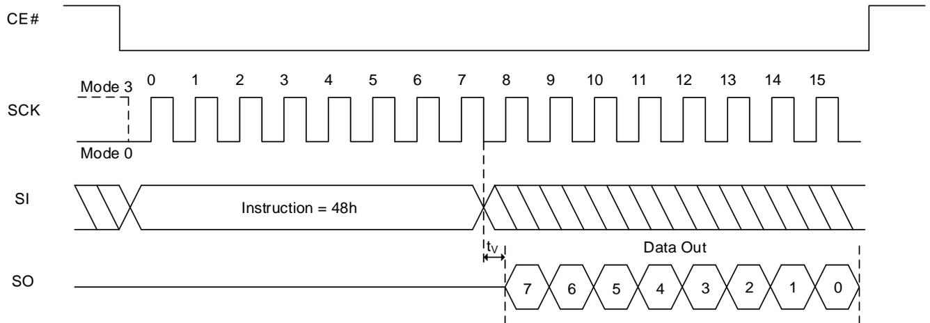
**Figure 8.28 Read Function Register Sequence In QPI Mode**
