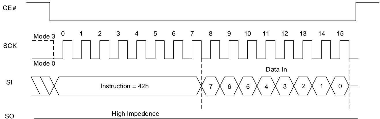
**Figure 8.30 Write Function Register Sequence In QPI Mode**
