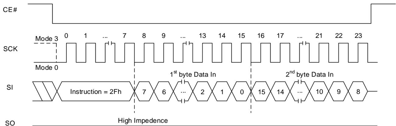
**Figure 8.87 Program ASP Sequence In QPI Mode**
