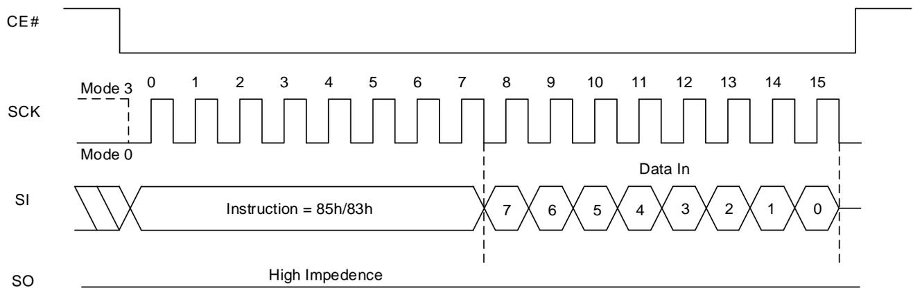
**Figure 8.40 Set Extended Read Parameters Sequence In QPI Mode**
