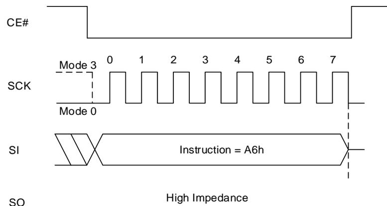
**Figure 8.90 Write PPB Lock Bit Sequence In QPI Mode**
