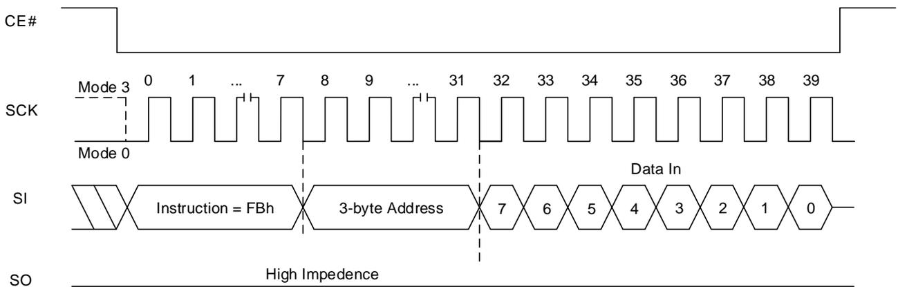
Figure 8.78 Write DYB Sequence In QPI Mode (FBh)
