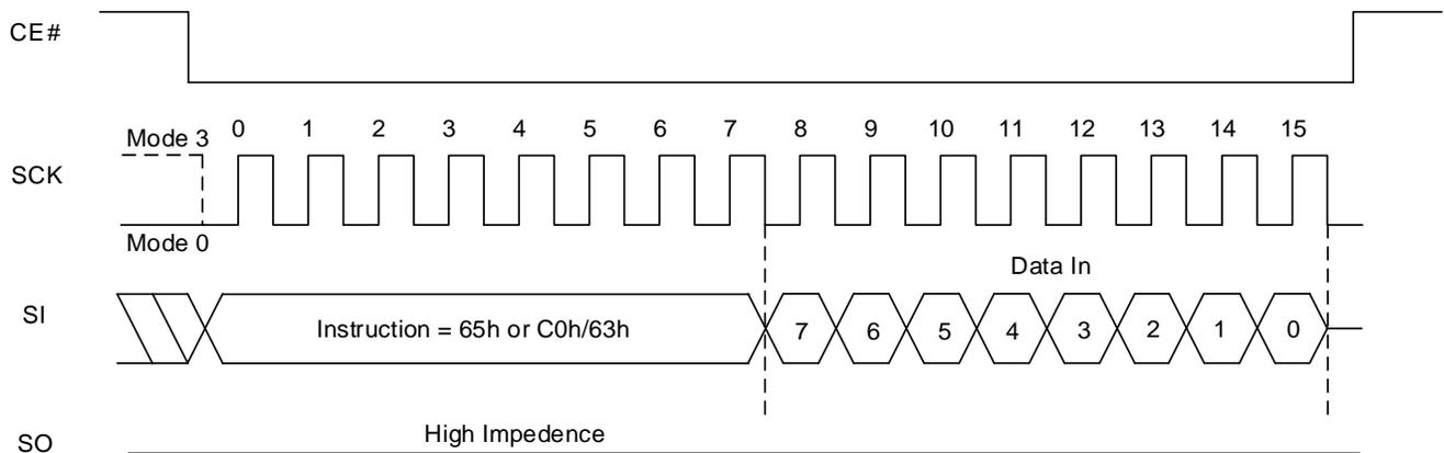
**Figure 8.38 Set Read Parameters Sequence In QPI Mode**
