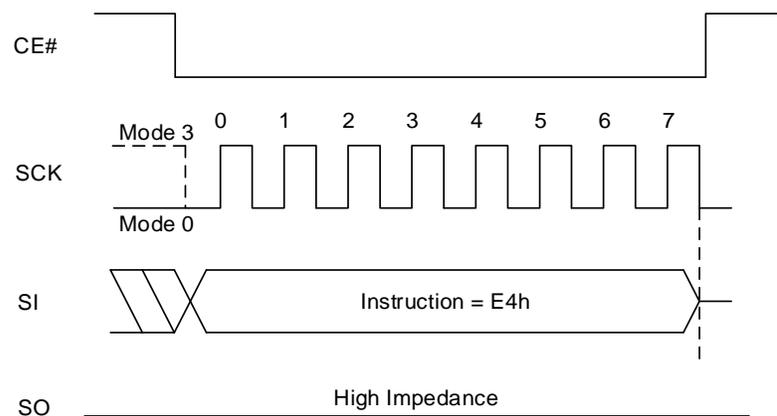
**Figure 8.83 Erase PPB Sequence In QPI Mode**
