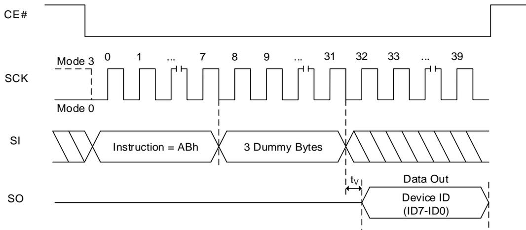
**Figure 8.48 Read Product Identification Sequence In QPI Mode**
