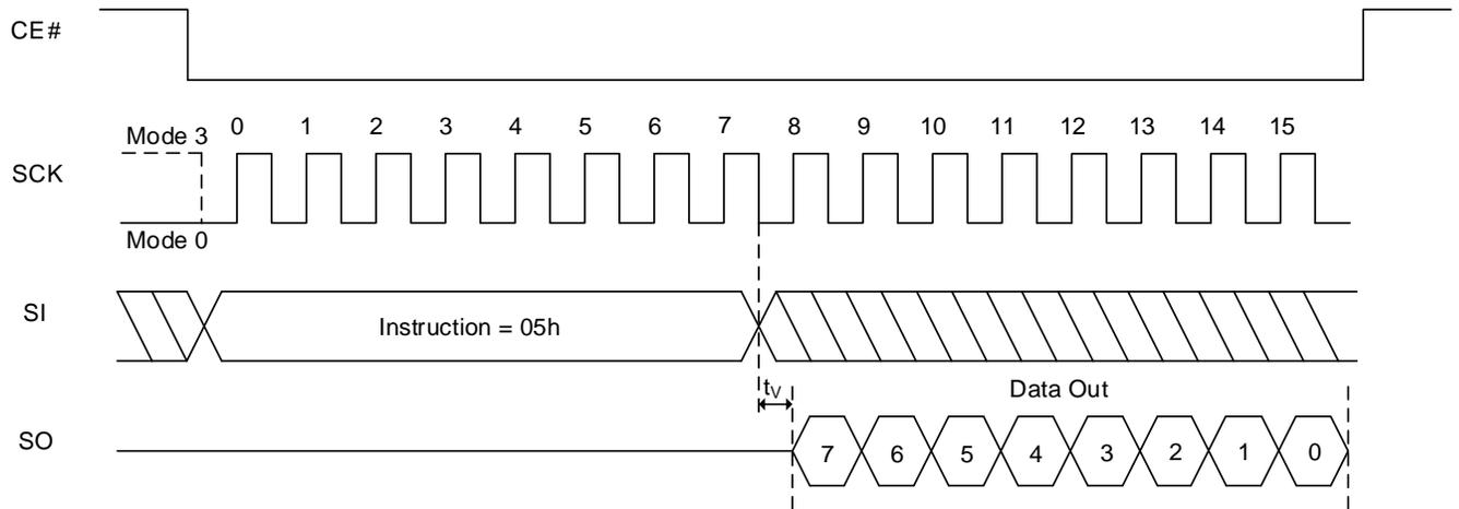
**Figure 8.24 Read Status Register Sequence In QPI Mode**
