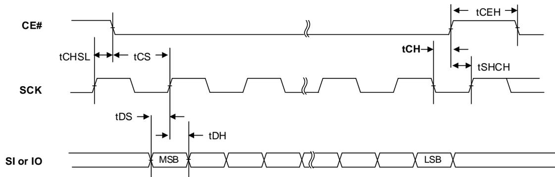
Figure 9.4 OUTPUT TIMING (STR Mode)
