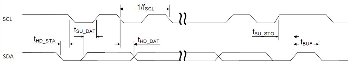
Figure 113: TWI timing diagram, 1 byte transaction
