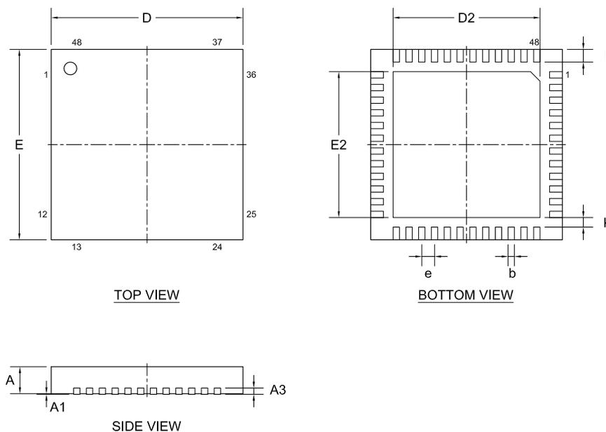
Figure 140: QFN48 6 x 6 mm package
