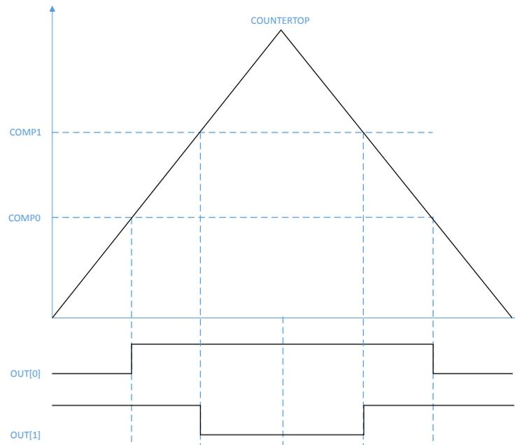
Figure 49: PWM counter in up-and-down mode example
