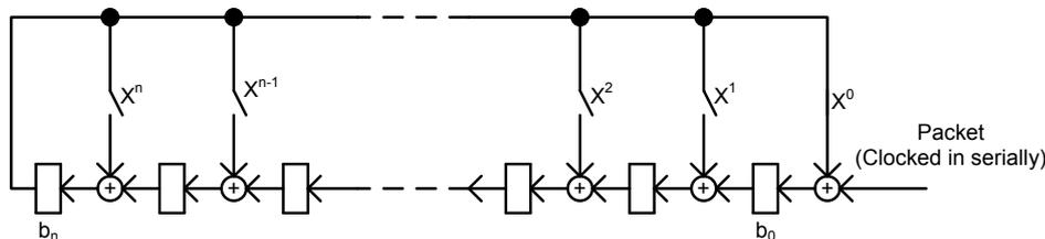
Figure 61: CRC generation of an  $n$  bit CRC
