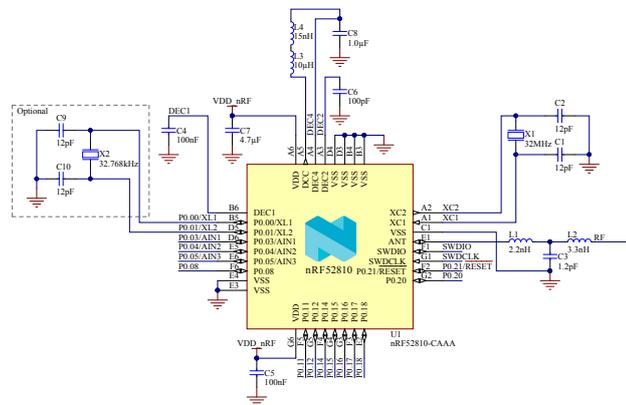
Figure 148: CAAA WLCSF with DC/DC regulator setup
