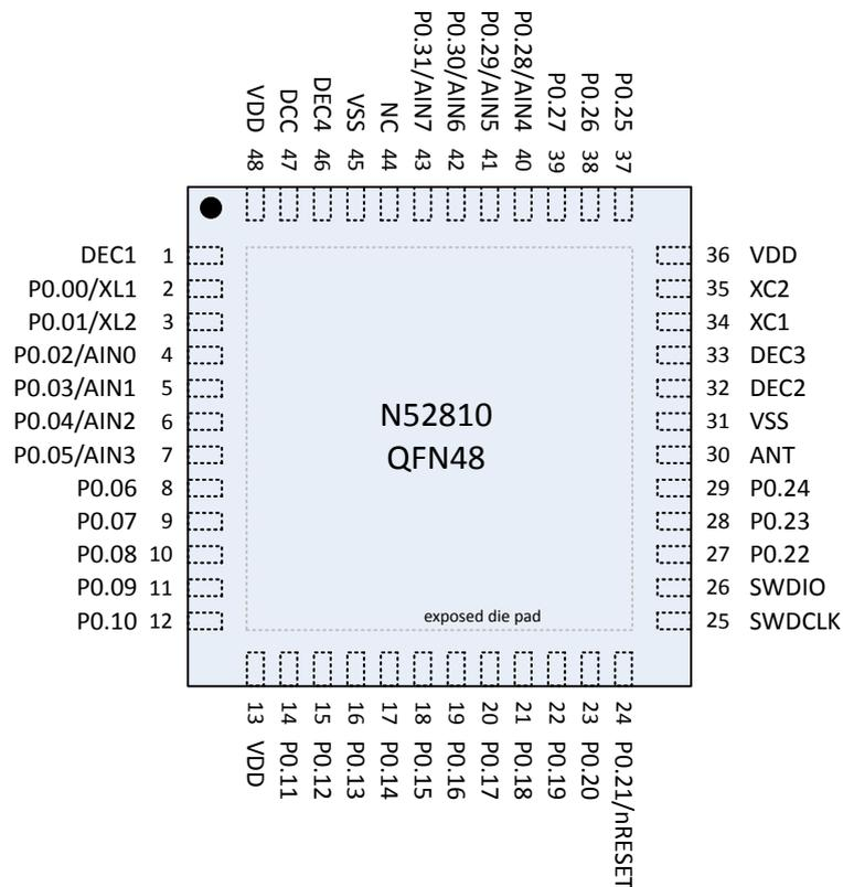
Figure 137: QFN48 pin assignments, top view
