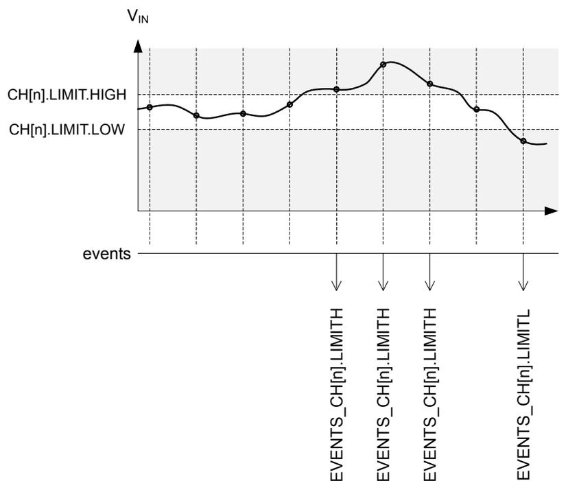
Figure 96: Example of limits monitoring on channel 'n'
