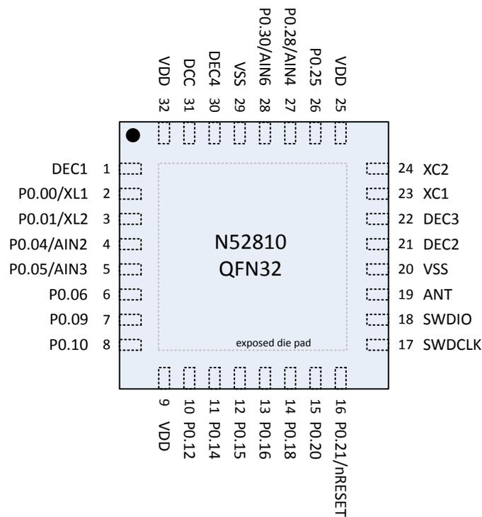
Figure 138: QFN32 pin assignments, top view
