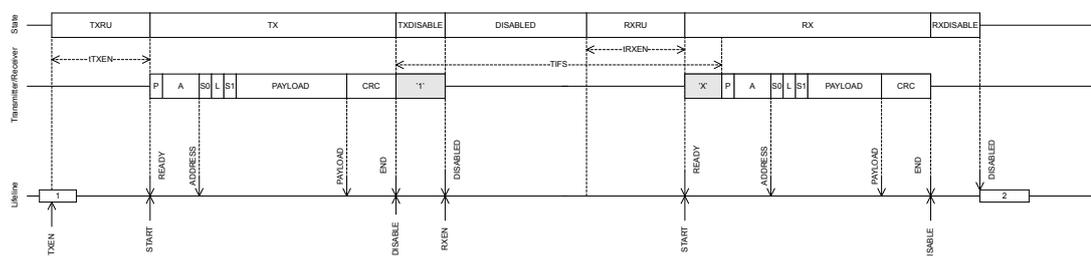
Figure 69: Ramp up and TIFS Timing Details
