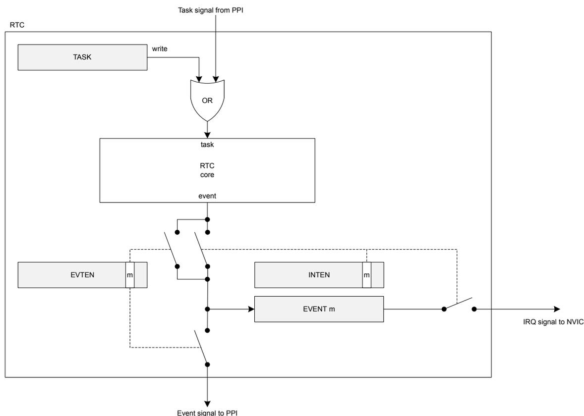
Figure 78: Tasks, events and interrupts in the RTC
