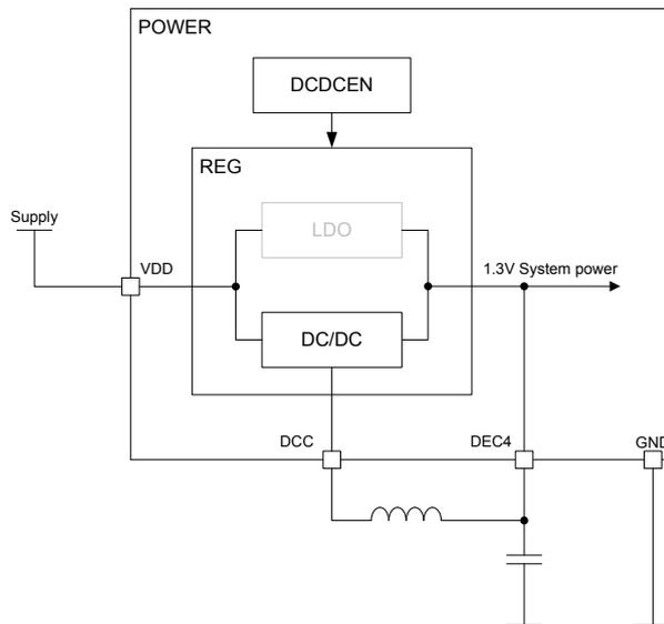
Figure 14: DC/DC regulator setup
