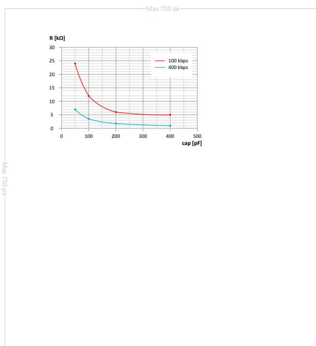
Figure 122: Recommended TWIM pullup value vs. line capacitance
