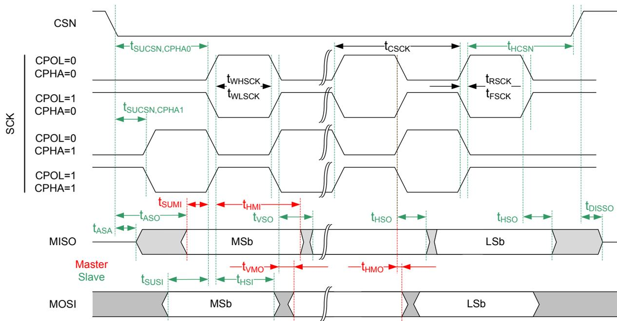
Figure 107: Common SPIM and SPIS timing diagram
