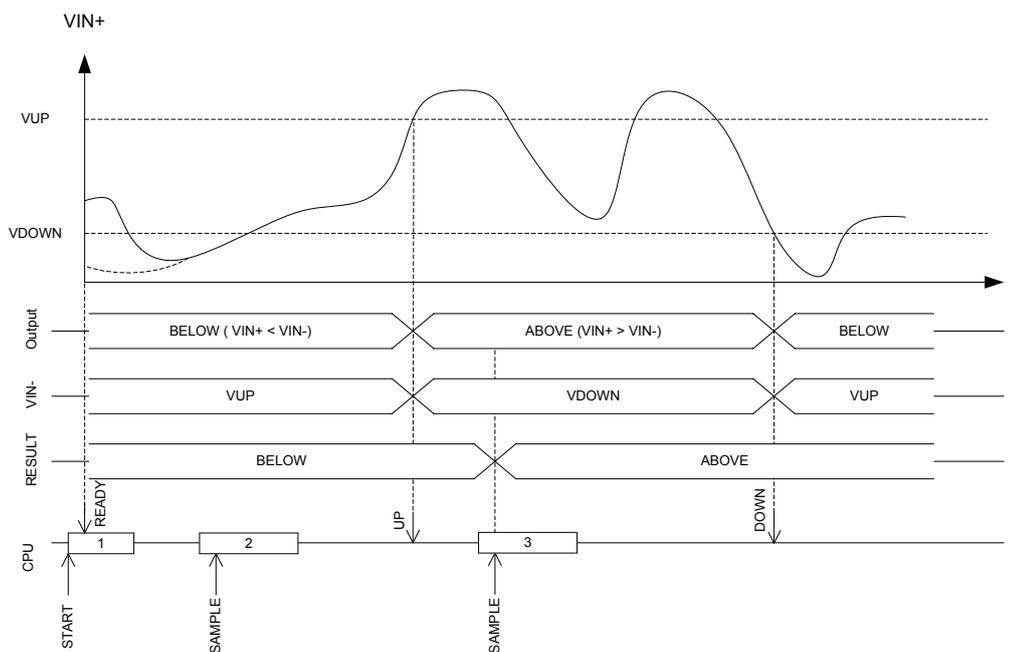
Figure 37: Hysteresis example where  $VIN+$  starts below  $VUP$
