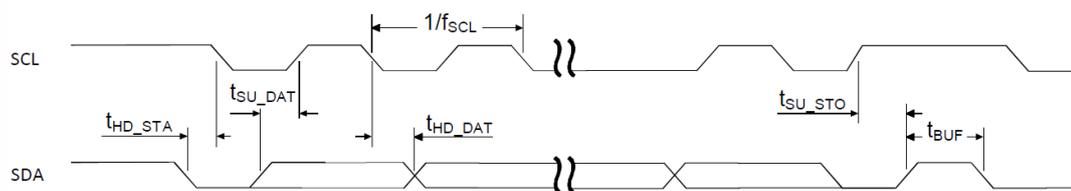
Figure 129: TWIS timing diagram, 1 byte transaction
