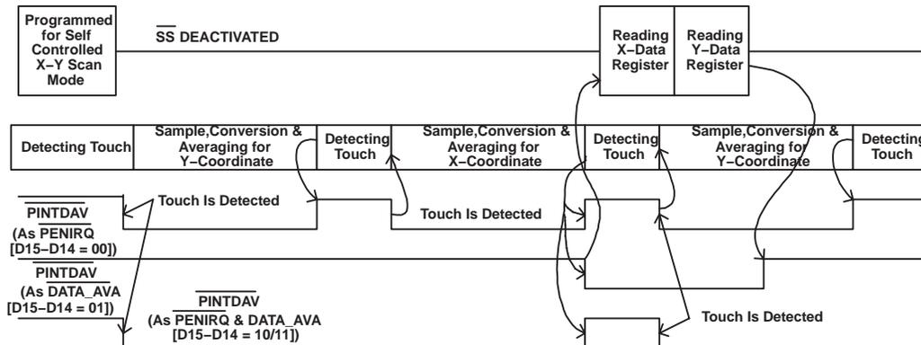
The time for a complete X/Y/Z1/Z2 coordinate conversion is given by (not including the time needed to send the command over the SPI bus):
