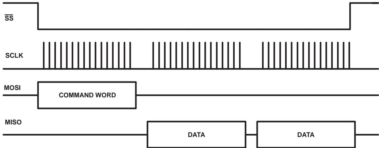
Figure 25. Read Operation for TSC2102 SPI Interface
