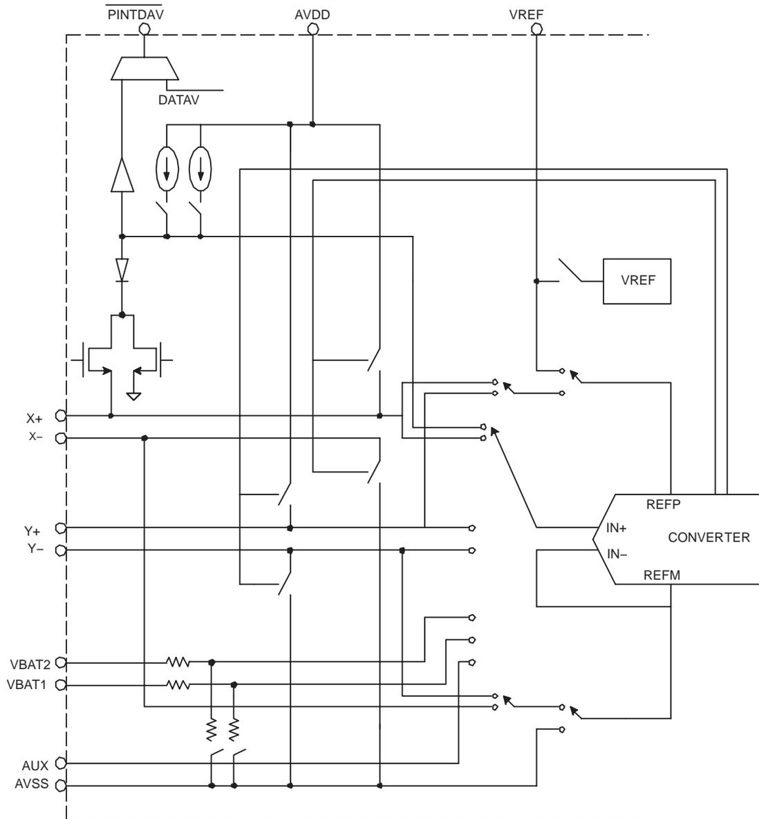
**Figure 12. Simplified Diagram of the Analog Input Section**
