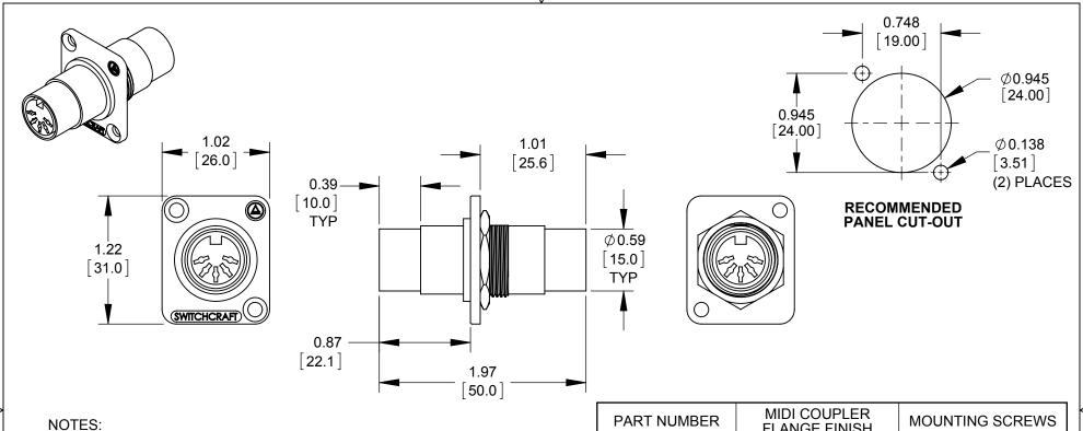
1. MATERIALS: MIDI COUPLER: **BODY - BRASS, NICKEL PLATED INSULATION - THERMOPLASTIC** NUT - BRASS, NICKEL PLATED MIDI COUPLER FLANGE - ZINC ALLOY, SEE TABLE FOR FINISH
